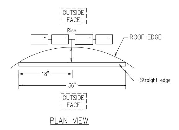
INDICATE PROPER RADIUS CONDITION BY NOTE! CIRCLING APPROPIATE OUTSIDE FACE.
