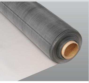
Versico Roofing Systems' VersiGard Cool Gray EPDM is a 60-mil non-reinforced roof membrane. It may be used for new construction and re-roofing applications and is available in a 10' x 100' roll. VersiGard Cool Gray EPDM is a game changer and the only EPDM membrane in the market ideal for locations where heating and cooling days are equal.
