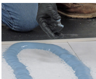
Performing the string-time test
