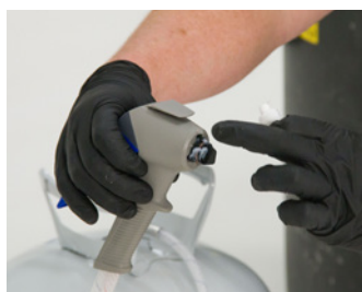
Application of petroleum jelly to spray gun
