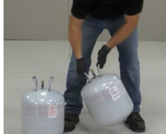
Shaking of A-side and B-side tanks
