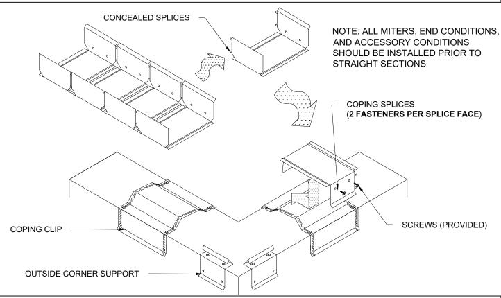
STEP 4: LOCATE MITER AND PLACE ONE LEG OVER THE CORNER SUPPORT AND CLIP, ROTATE BACKWARD AND PRESS DOWNWARD ON CAP TO ENGAGE ONTO CLIP, THEN REPEAT ON ADJACENT LEG OF MITER. (INSIDE MITER IS INSTALLED IN THE SAME MANNER USING INSIDE CORNER SUPPORTS).
