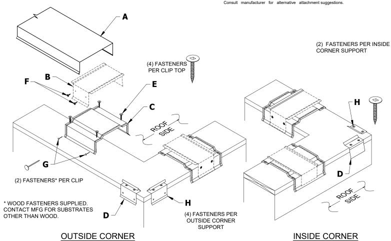
NOTE: ALL MITERS, END CONDITIONS, AND ACCESSORY CONDITIONS SHOULD BE INSTALLED PRIOR TO STRAIGHT SECTIONS
