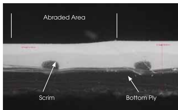
Membrane: 60-mil PVC Beginning Thickness: 59.77 Ending Thickness: 54.81
