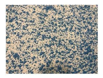
FIG 1. CORRECT COVERAGE - SPLATTER **APPLICATION**
