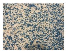
Fig 3. Correct Coverage – Splatter Application
