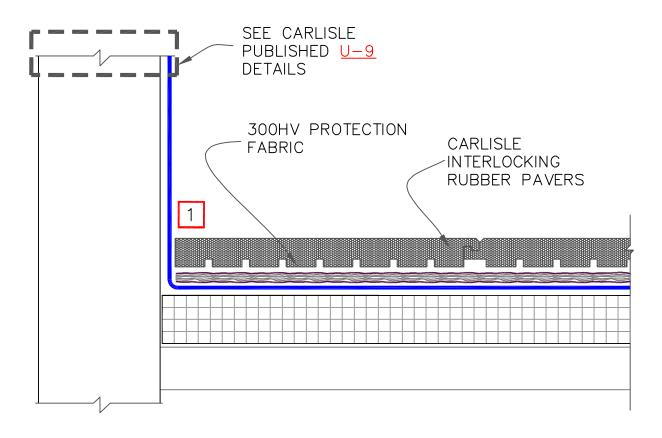
1. RUBBER PAVERS SHOULD BUTT TIGHTLY TO PARAPET WALLS. REFER TO CARLISLE'S RUBBER PAVER INSTALLATION GUIDE FOR MORE INFORMATION.
