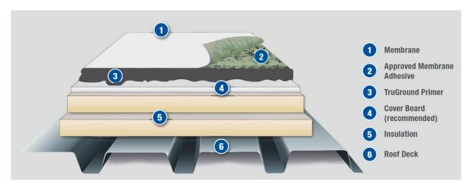
**Typical Roof Assembly with Conductive Primer**
