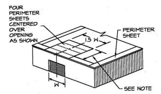
3) As an option to the above perimeter securement, an adhered membrane section
