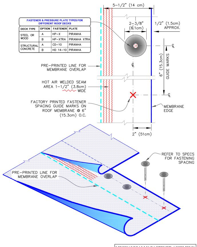
MECHANICALLY FASTENED ASSEMBLY
