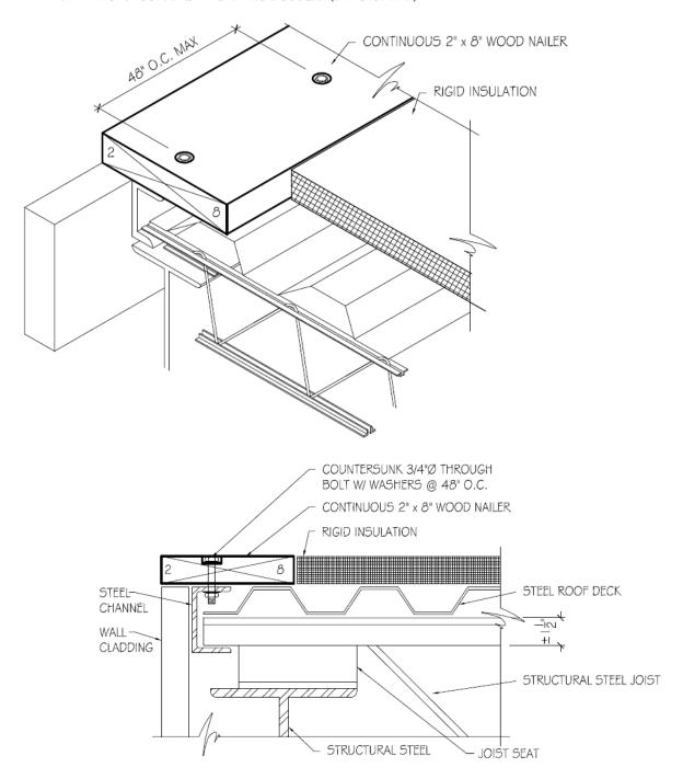
FIGURE 4 - ROOF EDGE WOOD BLOCKING - THROUGH BOLT ANCHORS
