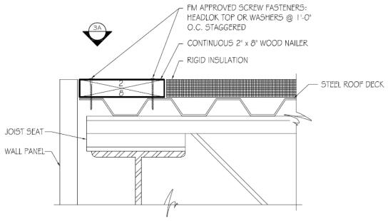
FIGURE 2 - ROOF EDGE WOOD BLOCKING - SCREW FASTENER ANCHORAGE
