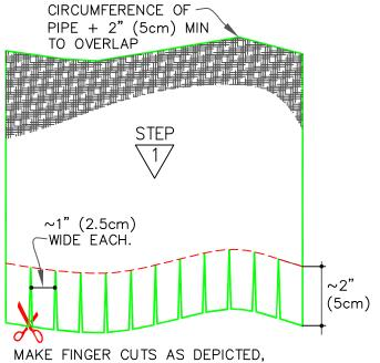
APPLY BASE COAT OF LIQUISEAL Liquid Flashing Resin PER PUBLISHED COVERAGE RATE STEP 1
