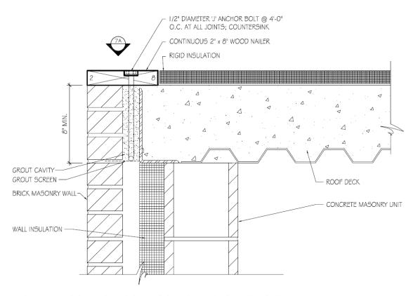
FIGURE I - ROOF EDGE WOOD BLOCKING - ANCHOR BOLT SECUREMENT
