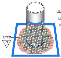
IMMEDIATELY PRESS LIQUISEAL Flashing Fleece, INTO THE APPLIED LIQUISEAL Liquid Flashing Resin. APPLY SECOND COAT OF RESIN. ENSURE ALL ENDS OF FINGERS ARE PROPERLY EMBEDDED.
