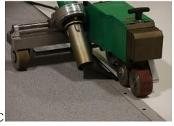
WELD TPO OR PVC MEMBRANE TO COATED METAL STRIP.
