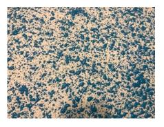
Fig 3. Correct Coverage – Splatter Application
