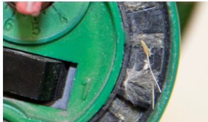
Dirt and debris in intake
