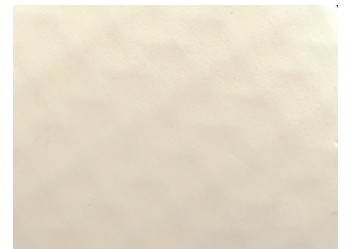
Versico VersiWeld TPO – 60 Weeks (No Failure)
