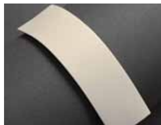
Versico VersiWeld TPO – 60 Weeks (No Failure)
