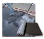
A 90-mil SBS-modified asphalt base sheet. Can be used in multi-ply roofing systems as an air and vapor barrier, or as a temporary roof for up to 60 days. This product is fiberglass-reinforced and meets or exceeds requirements of ASTM 6363 Type 1. When used as an air and vapor barrier, suitable substrates include concrete (primer required), DensDeck Prime, and SECUROCK.
