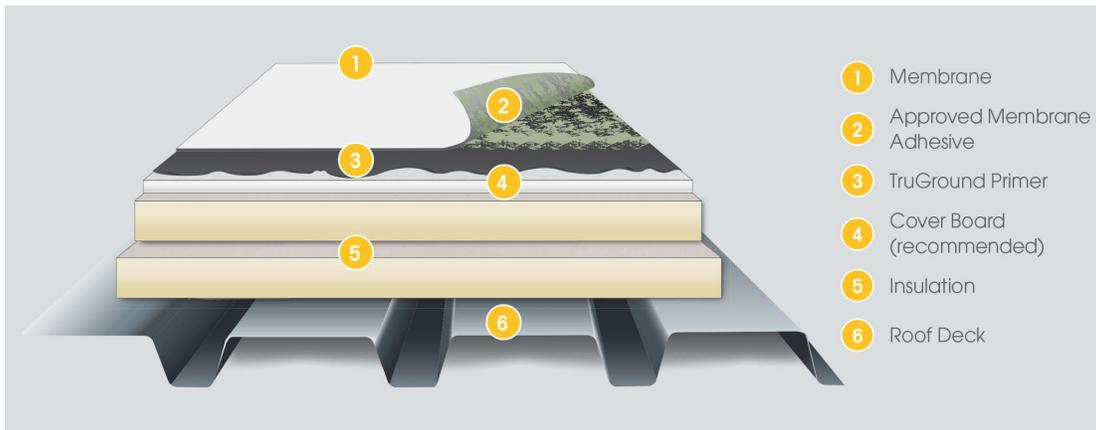
**Typical Roof Assembly with Conductive Primer**
