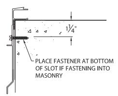
PLACE FASTENER AT BOTTOM OF SLOT IF FASTENING INTO ELIMINAILER<sub>0</sub>-T
