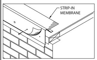
3. POSITION STRIP-IN MEMBRANE OVER AND DOWN WATERDAM FACE APPROXIMATELY 1" BELOW RAISED FASTENING HOLES (PROVIDED). TAKE CARE TO AVOID BRIDGING OF MEMBRANE. LOCATE AND FASTEN MEMBRANE AT 12" O.C. THROUGH ALL RAISED HOLES ON OUTSIDE FACE USING PROVIDED FASTENERS.
