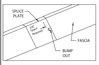
5. INSTALL 12'-0" FASCIA COVER SECTIONS. INSERT ONE SPLICE PLATE UNDER EACH OF THE FASCIA COVERS. INSTALL COVER BY PUSHING DOWNWARD UNTIL FASCIA COVER IS ENGAGED TO WATER DAM ALONG ENTIRE LENGTH. CONTINUE TO INSTALL FASCIA COVERS, FIELD CUTTING WHERE NECESSARY USING FINE TOOTH HACKSAW.
