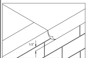
1. POSITION MEMBRANE OVER THE ROOF EDGE AND DOWN OUTSIDE FACE OF WALL, COVERING TREATED WOOD NAILER(S) COMPLETELY. ALLOW 1/3" EXCESS MFMBRANF.
