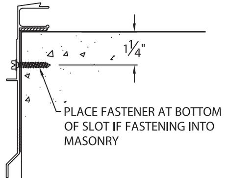
PLACE FASTENER AT BOTTOM OF SLOT IF FASTENING INTO ELIMINAILER-T
