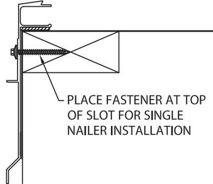
PLACE FASTENER AT BOTTOM OF SLOT IF 1/2" COVER BOARD IS USED
