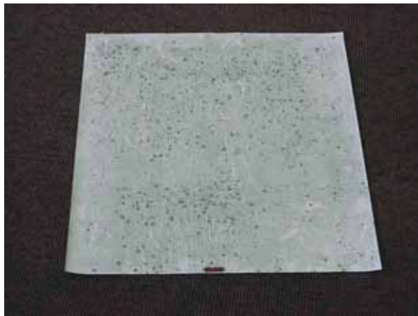
PVC membrane with a lacquer-coated top ply
