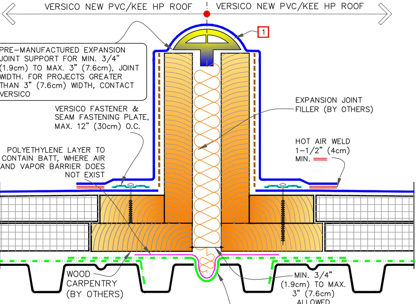
ROOF AIR & VAPOR RETARDER WHERE REQUIRED. DO NOT REMOVE LINER IN EXPOSED AREAS AT JOINT.
