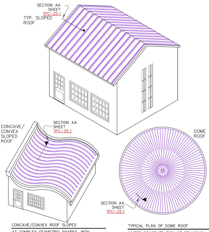
AT COMPLEX GEOMETRIC SHAPES, WITH MULTI-DIRECTIONAL SLOPES, THE SHEET METAL ROOF IS NOT ONLY DIFFICULT TO INSTALL, BUT THE WATER-SHEDDING ABILITY OF METAL ROOF IS SERIOUSLY HAMPERED WITHIN THE CONCAVE (NEGATIVE) SLOPES. THE WATERPROOFED ROOF MEMBRANE WITH THE CONTOUR RIB IS A PRACTICAL SOLUTION.
