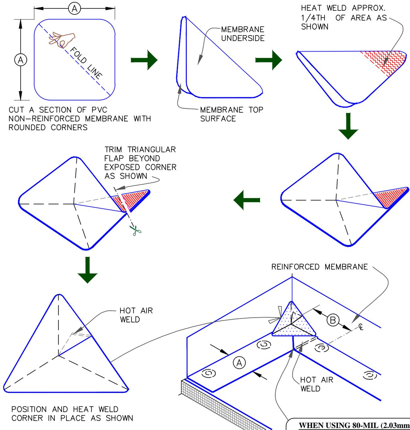
**WHEN USING 80-MIL (2.03mm) THICK MEMBRANE**
