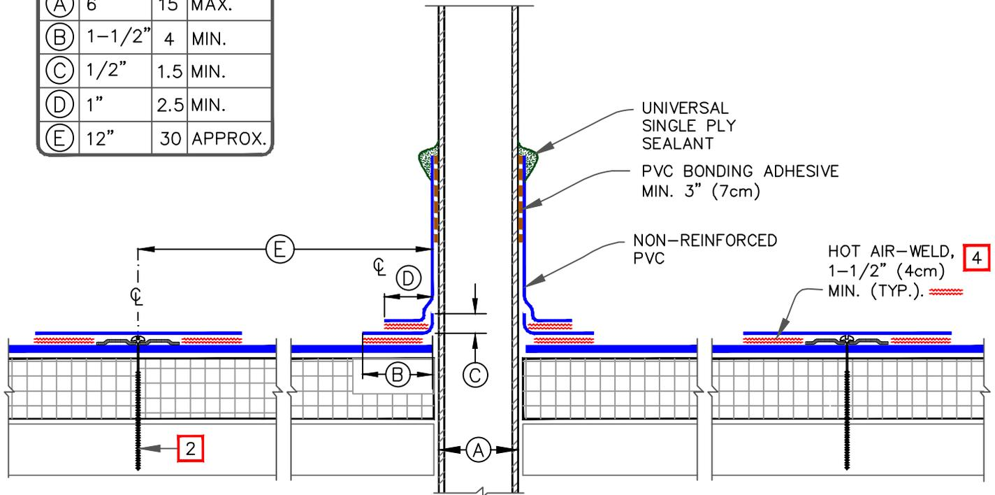
**FASTENER TYPES ON MECHANICALLY ATTACHED ROOF ASSEMBLY**
