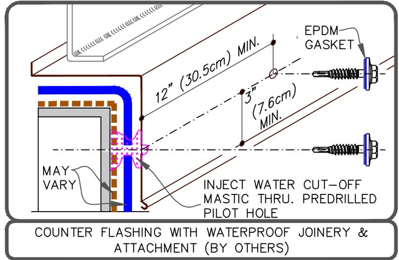
PVC ONLY (NOT KEE HP) IN LIEU OF BONDING ADHESIVE, THE CURB FLASHING MAY BE INSTALLED IN CAV GRIP PVC.
