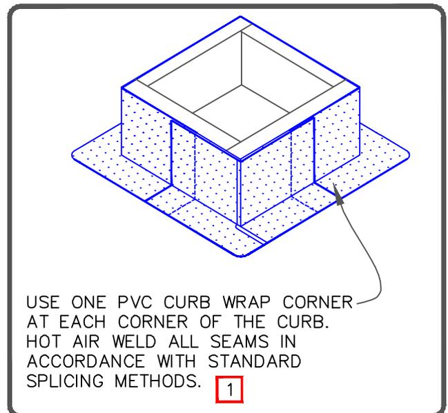
USE ONE PVC CURB WRAP CORNER AT EACH CORNER OF THE CURB. HOT AIR WELD ALL SEAMS IN ACCORDANCE WITH STANDARD SPLICING METHODS. **1**
