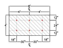
FIELD OF ROOF 6 FASTENERS PER 4'X8' BOARD
