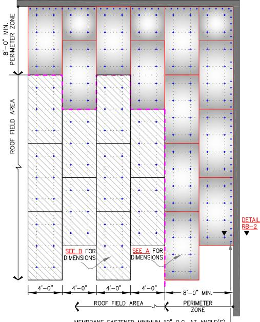
MEMBRANE FASTENED MINIMUM 12" O.C. AT ANGLE(S)-CHANGES. FOR ADDITIONAL INFORMATION SEE DETAIL  $\frac{RB-2}{}$
