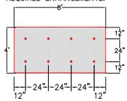
PERIMETER ZONE 8 FASTENERS PER 4'X8' BOARD
