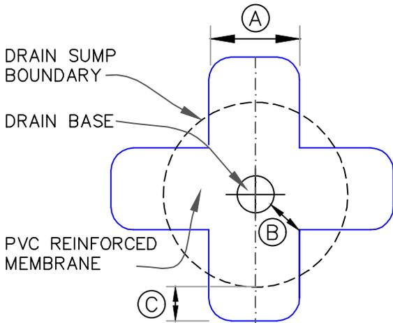
CUT SECTION OF PVC REINFORCED MEMBRANE AS SHOWN AND POSITION INTO DRAIN SUMP. EXTEND MEMBRANE OUT OF DRAIN SUMP APPROXIMATELY 6" (15cm) (ROUND CORNERS).
