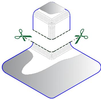
60-MIL (1.52mm) THICK PVC, UNIVERSAL CORNER CAN BE USED FOR AT TOP CORNER. CUT AS SHOWN IN DETAIL [TPC-15.7](#)
