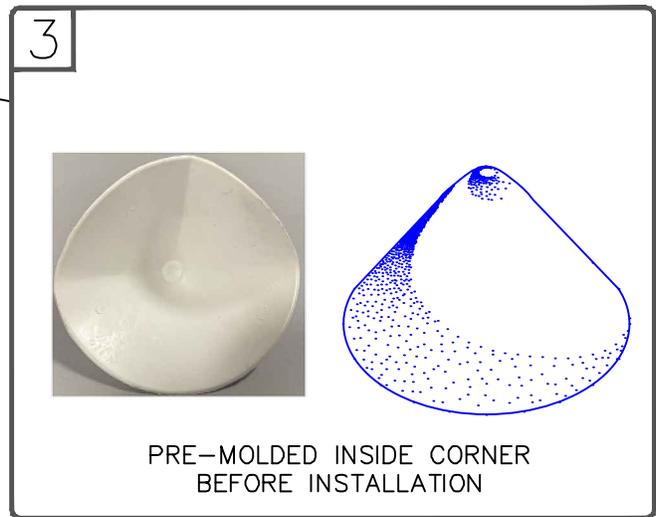
**WHEN USING 80-MIL (2.03mm) THICK MEMBRANE**
