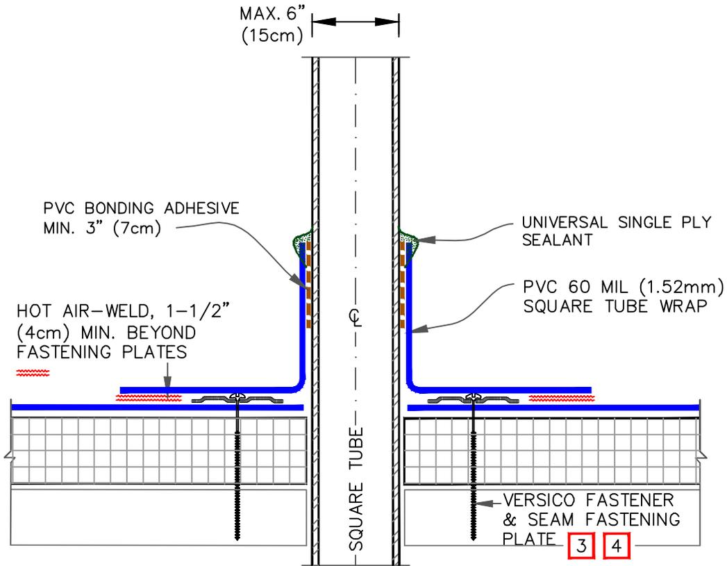
**FASTENER TYPES ON MECHANICALLY ATTACHED ROOF ASSEMBLY**
