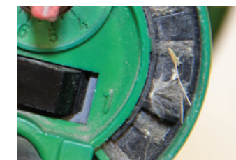
DIRT AND DEBRIS IN INTAKE
