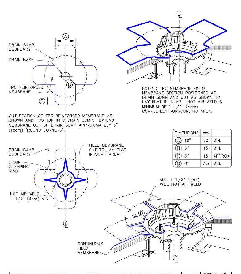
ROOF DRAIN: SUMP SLOPE GREATER THAN 3" TO 1" HORIZONTAL FOOT (OPTION 2), PAGE 2 OF 2
