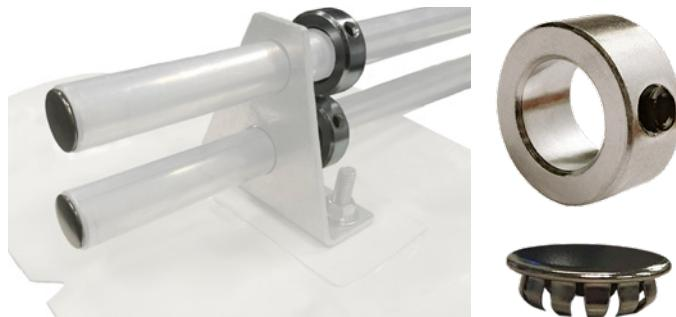
The Snow Retention Pipes are secured in place with pipe collars, which are tightened onto the pipes using the provided set screws. Position each collar approximately 1" to 2" inside the first and last mounting brackets. The collars prevent the pipes from shifting or slipping out of the brackets. End caps are installed in the exposed pipe ends to provide a clean, finished appearance.
