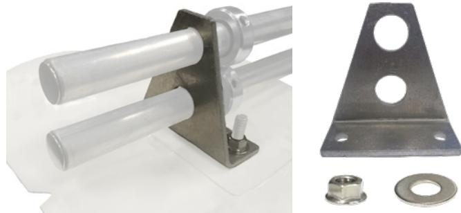
The snow retention system is attached to the U3400 anchors using the mounting brackets along with the supplied washers and flange nuts. Tighten and torque the flange nuts to approximately 20 to 25 ft-lbs to ensure the brackets are properly secured.
