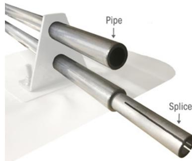
The Snow Retention Pipes have a 1" outside diameter and are supplied in 8' lengths. Insert the pipes into the mounting brackets. For runs longer than 8', splices are available to connect adjacent pipes; however, splices must not be located within 6" of a bracket. Continuous runs of snow retention pipe must not exceed 100'. For runs exceeding 100', introduce a short break and begin a new assembly along the same line to accommodate thermal expansion and contraction.
