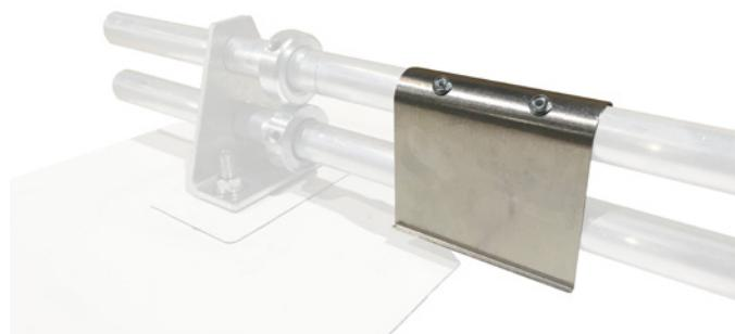
Restrictor plates are an optional component installed on the top pipe of the snow retention system. Each plate extends downward beyond the bottom pipe, closer to the membrane, to help prevent smaller snowfalls from sliding beneath the system. The quantity and spacing of restrictor plates should be determined by the system designer.
