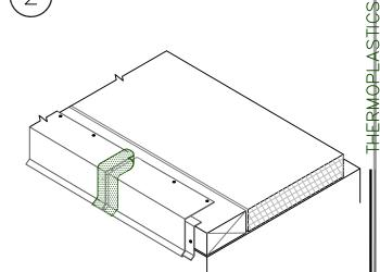
HEAT WELD 3" (7.5cm) WIDE PIECE OF NON-REINFORCED THERMOPLASTIC MEMBRANE OVER JOINT.
