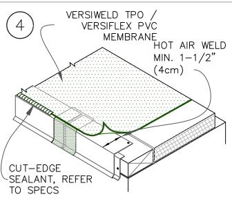
POSITION FIELD MEMBRANE AND HEAT WELD TO COATED METAL A MINIMUM OF 1-1/2" (4cm) AS SHOWN.
