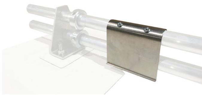
Restrictor plates are an optional component installed on the top pipe of the snow retention system. Each plate extends downward beyond the bottom pipe, closer to the membrane, to help prevent smaller snowfalls from sliding beneath the system. The quantity and spacing of restrictor plates should be determined by the system designer.
