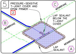
APPLY PRESSURE—SENSITIVE T—JOINT COVER OR 6" (15cm) WIDE SECTION OF PRESSURE—SENSITIVE ELASTOFORM FLASHING CENTERED OVER THE INTERSECTING POINT OF THE LEADING EDGES OF THE FIELD SPLICE INTERSECTION AS SHOWN.
