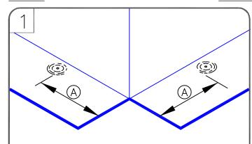
FASTEN MEMBRANE AND FLASH CURB OR WALL WITH CURED EPDM MEMBRANE FOLLOWING STANDARD PROCEDURES USING BONDING ADHESIVE and SecurTAPE.
