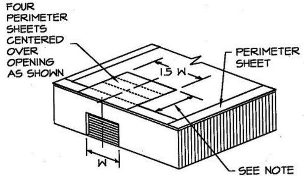
3) As an option to the above perimeter securement, an adhered membrane section may be used in lieu of the mechanically fastened membrane at large openings in accordance with the Carlisle Specification for the Sure-Seal/Sure-White Adhered Roofing System.
