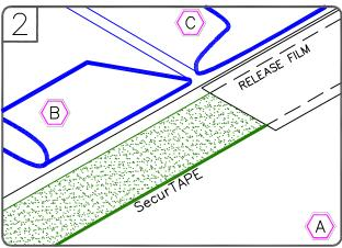
FOLD SHEETS BACK AS SHOWN. APPLY EPDM PRIMER TO THE SPLICE AREA ON BOTH SURFACES AND ALLOW TO FLASH—OFF. APPLY SecurTAPE WITH RELEASE FILM ALIGNED WITH MARKED LINE.
