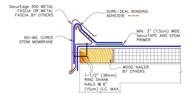
1. 6" (15cm) WIDE PRESSURE—SENSITIVE ELASTOFORM FLASHING, IN CONJUNCTION WITH EPDM PRIMER, MUST BE CENTERED OVER FIELD SPLICES AT THE ANGLE CHANGE.
