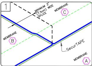
POSITION MEMBRANE TO ALLOW AN APPROXIMATE 4" (10cm) OVERLAP. MARK THE BOTTOM SHEET WITH AN INDELIBLE MARKER 1/2" (1.5cm) FROM THE EDGE OF THE TOP SHEET AS SHOWN. THE PRE-MARKED LINE ON THE MEMBRANE EDGE CAN ALSO BE USED AS A GUIDE.
