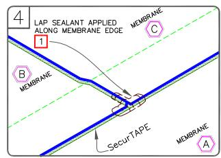
SPLICE SHEET C TO SHEET A AND B, PRESS TOP SHEET ONTO BOTTOM SHEET USING HAND PRESSURE TOWARDS THE OUTER EDGE OF THE SPLICE AND ROLL THE SPLICE AREA WITH A 2" (5cm) WIDE STEEL ROLLER.
