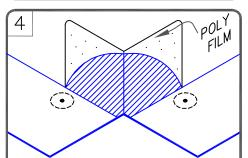
REMOVE & REPLACE POLY BACKING ON FLASHING. FOLD FLASHING IN HALF WITH ROUNDED PORTION TURNED UP. CENTER ON CORNER & FIRMLY PRESS AGAINST VERTICAL **SURFACE**
