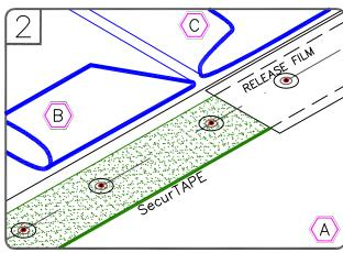
FOLD SHEETS BACK AS SHOWN. APPLY EPDM PRIMER TO THE SPLICE AREA ON BOTH SURFACES AND ALLOW TO FLASH-OFF. SecurTAPE WITH RELEASE FILM ALIGNED WITH PRE-MARKED LINE.
