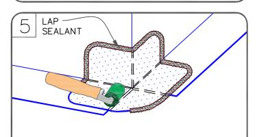
AFTER ADHERING, ROLL WITH A TWO INCH WIDE STEEL HAND ROLLER. PAY PARTICULAR ATTENTION TO THE STEP OFFS AND ANGLE CHANGES.
