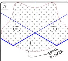
CLEAN EPDM SPLICE AREA WITH WEATHERED MEMBRANE CLEANER PRIOR TO APPLYING EPDM PRIMER
