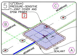
APPLY 6"(15cm) PRESSURE-SENSITIVE T-JOINT COVER AND 12"(30cm) PRESSURE-SENSITIVE T-JOINT COVER OR PRESSURE-SENSITIVE ELASTOFORM CENTERED OVER THE INTERSECTING POINT OF THE LEADING EDGES OF THE FIELD SPLICE INTERSECTION AS SHOWN.
