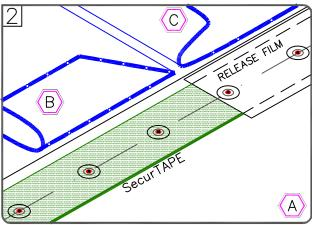
FOLD SHEETS BACK AS SHOWN. APPLY EPDM PRIMER TO THE SPLICE AREA ON BOTH SURFACES AND ALLOW TO FLASH—OFF. APPLY SecurTAPE WITH RELEASE FILM ALIGNED WITH PRE—MARKED LINE.
