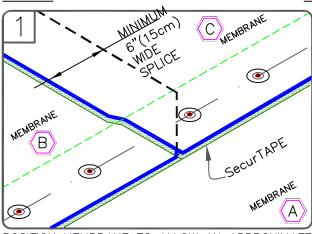
POSITION MEMBRANE TO ALLOW AN APPROXIMATE (17.5cm) OVERLAP. THE PRE-MARKED LINE ON THE MEMBRANE EDGE CAN BE USED AS A GUIDE FOR TAPE PLACEMENT.
