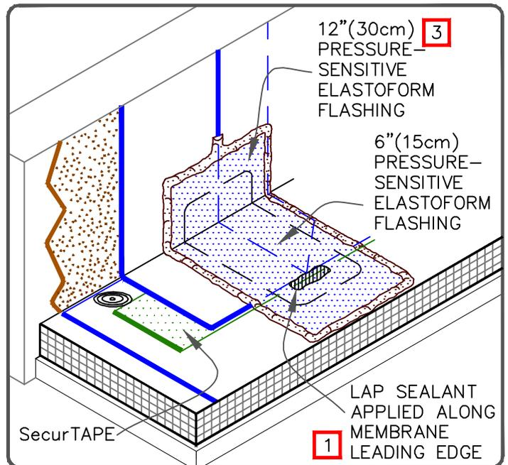
CONTINUOUS WALL FLASHING
