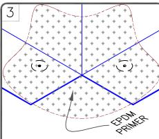
CLEAN EPDM SPLICE AREA WITH WEATHERED MEMBRANE CLEANER PRIOR TO APPLYING EPDM PRIMER
