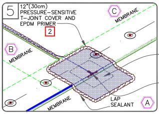
APPLY 6"(15cm) PRESSURE-SENSITIVE T-JOINT COVER AND 12"(30cm) PRESSURE-SENSITIVE T-JOINT COVER OR PRESSURE-SENSITIVE ELASTOFORM CENTERED OVER THE INTERSECTING POINT OF THE LEADING EDGES OF THE FIELD SPLICE INTERSECTION AS SHOWN.
