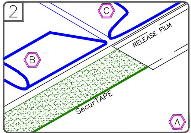
FOLD SHEETS BACK AS SHOWN. APPLY EPDM PRIMER TO THE SPLICE AREA ON BOTH SURFACES AND ALLOW TO FLASH-OFF. APPLY SecurTAPE WITH RELEASE FILM ALIGNED WITH MARKED LINE.
