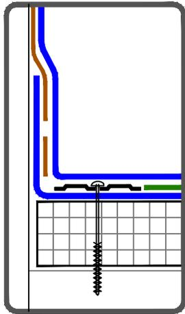
OPTIONAL: SEAM PLATE/FASTENER MAY BE INSTALLED INTO THE STRUCTURAL DECK UP TO 6" (15cm) FROM ANGLE CHANGE.
