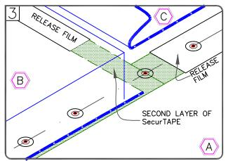
SPLICE SHEET B TO SHEET A AND APPLY SECOND PIECE OF SecurTAPE BETWEEN SHEET B AND C. TRIM RELEASE FILM AS SHOWN.
