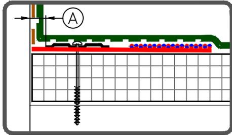
OPTIONAL: SEAM PLATE/FASTENER MAY BE INSTALLED INTO THE STRUCTURAL DECK UP TO 6" (15cm) FROM ANGLE CHANGE.
