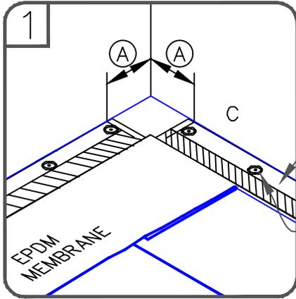
6" (15cm) WIDE PRESSURE-SENSITIVE RUSS (MAY BE FASTENED INTO VERTICAL SUBSTRATE)
