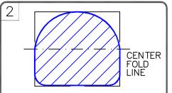
USE PRE-CUT T-JOINT COVERS OR CUT A 6"x6" (15X15cm) & 12"x12" (30X30cm) SECTION OF PRESSURE- SENSITIVE ELASTOFORM FLASHING AND ROUND CORNERS
