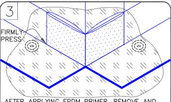
AFTER APPLYING EPDM PRIMER, REMOVE AND REPLACE POLY BACKING. FOLD FLASHING IN HALF WITH ROUNDED PORTION TURNED UP. CENTER FLASHING ON CORNER AND FIRMLY PRESS AGAINST VERTICAL SURFACE.
