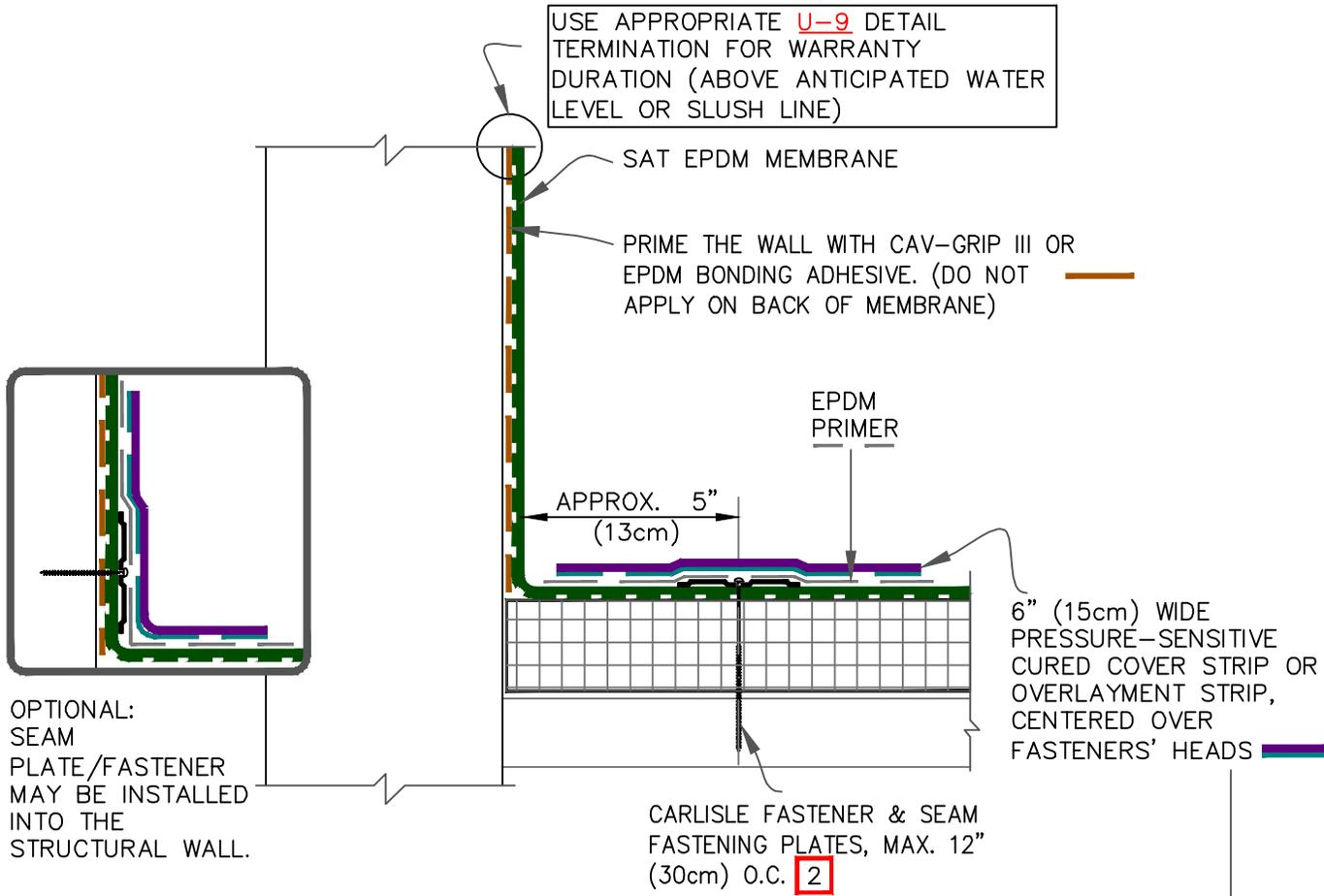
OPTIONAL: SEAM PLATE/FASTENER MAY BE INSTALLED INTO THE STRUCTURAL WALL.
