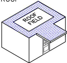
INSTALL PERIMETER SHEETS OVER THE ENTIRE OVERHANG AREA, EXTENDING ONTO THE MAIN ROOF DECK WHEN AT THE SAME LEVEL AS SHOWN.
