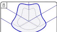
APPLY EPDM PRIMER TO SPLICE AREA. INSTALL THE 12"X12" (30cmX30cm) SECTION OF PRESSURE - SENSITIVE ELASTOFORM FLASHING CENTERED OVER PREVIOUSLY APPLIED FLASHING.
