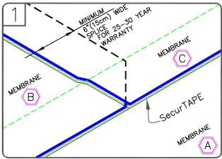
POSITION MEMBRANE TO ALLOW AN APPROXIMATE 7" (17.5cm) OVERLAP. MARK THE BOTTOM SHEET WITH AN INDELIBLE MARKER 1/2" (1.5cm) FROM THE EDGE OF THE TOP SHEET AS SHOWN. THE PRE-MARKED LINE ON THE MEMBRANE EDGE CAN ALSO BE USED AS A GUIDE.
