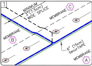
POSITION MEMBRANE TO ALLOW AN APPROXIMATE 7" (17.5cm) OVERLAP ALONG THE LENGTH OF THE MEMBRANE & 4" (10cm) AT END LAPS. THE PRE-MARKED LINE ON THE MEMBRANE EDGE CAN BE USED AS A GUIDE FOR TAPE PLACEMENT.
