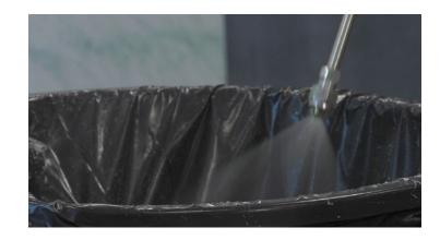
**Step 6:** Relieve the pressure in the hose by triggering the gun into the trash can. Remove any adhesive residue from the spray tip. Disconnect the hose from the UN-TACK cylinder. The gun and hose are now in a storable condition. It is a good idea to protect the hose end to eliminate contaminant entry.
