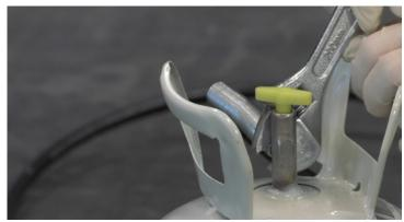
**Step 4:** Connect the hose to the UN-TACK cylinder using an open-end or adjustable wrench.
