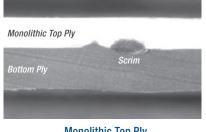
Monolithic Top Ply Features a 24-mil monolithic thickness over scrim. The entire top ply is a fully formulated polymer for maximum weatherability and long-term protection against the elements.
