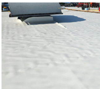
Dunnage marks on unrolled sheets and crushed cores due to over-stacking, dunnage, and wet cores due to not being covered
