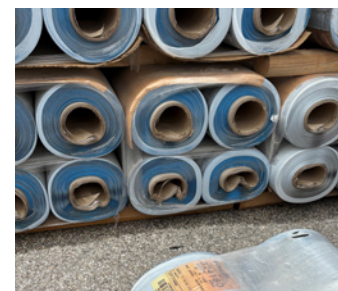
Dunnage marks on unrolled sheets and crushed cores due to over-stacking, dunnage, and wet cores due to not being covered
