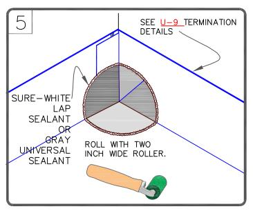
1. TPO PRIMER MUST BE APPLIED TO ALL SPLICE AREAS AND FOR EACH LAYER OF PRESSURE—SENSITIVE FLASHING.
