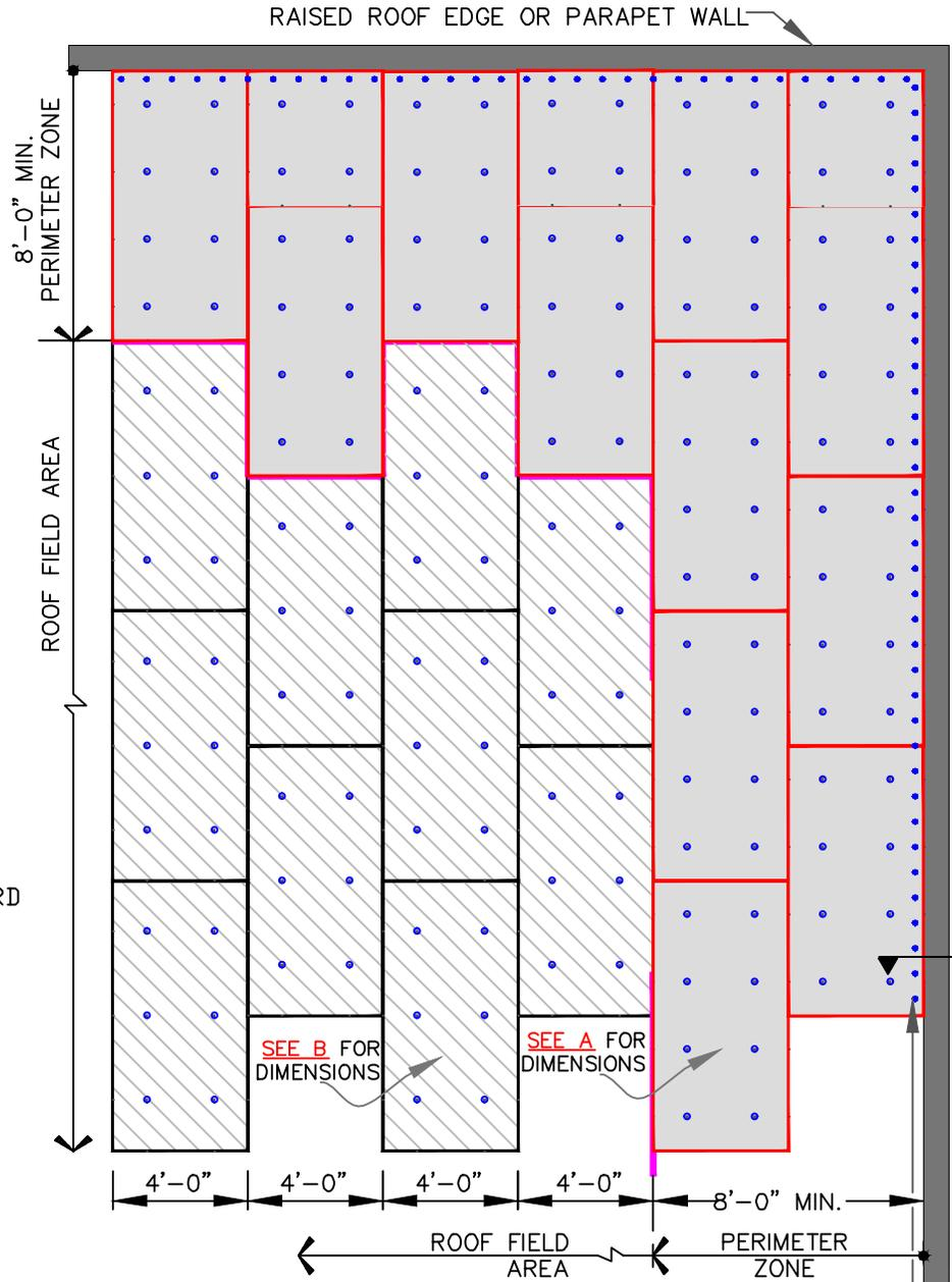
MEMBRANE FASTENED MINIMUM 12" O.C. AT ANGLE(S) CHANGES. FOR ADDITIONAL INFORMATION SEE DETAIL IW-2
