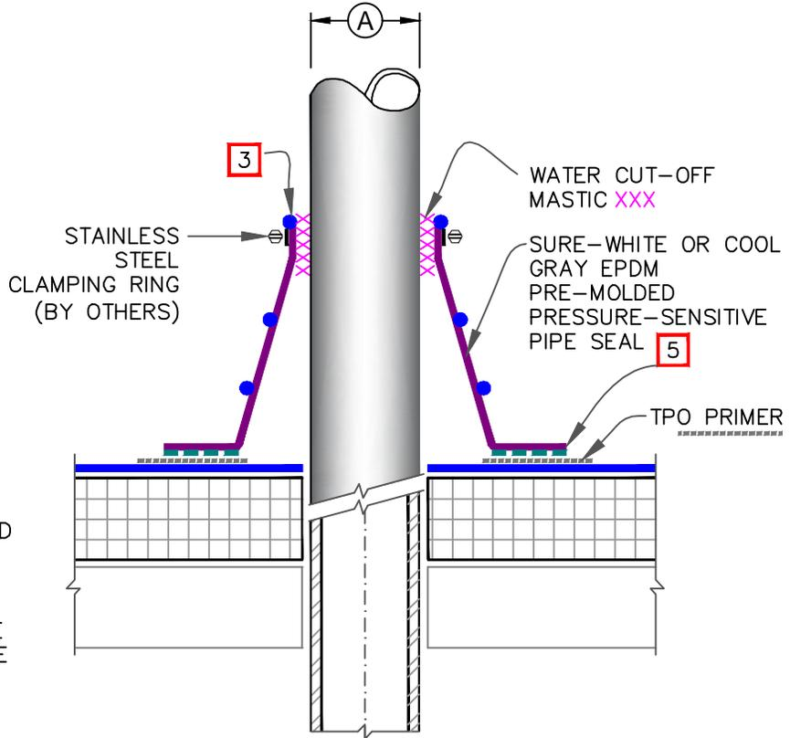
TPO WITH EPDM FLASHING
