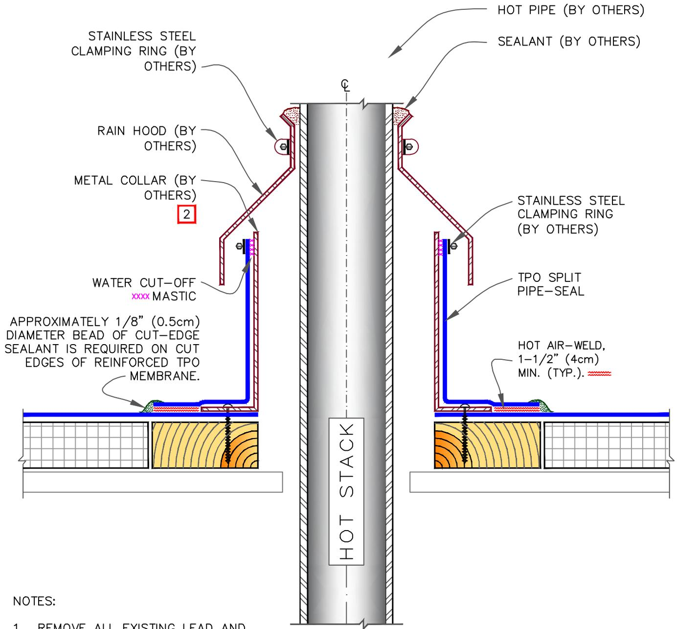
APPROXIMATELY 1/8" (0.5cm) DIAMETER BEAD OF CUT-EDGE SEALANT IS REQUIRED ON CUT EDGES OF REINFORCED TPO MEMBRANE.
