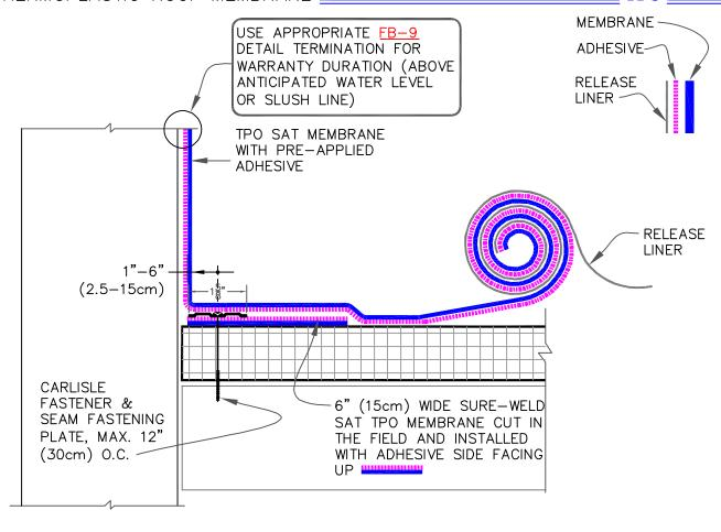
1. WIND SPEED GREATER THAN 90 MPH (145 KILOMETERS /HOURS)(40.3 METER PER SECOND) OR PROJECTS WITH 25 OR 30-YEAR WARRANTIES REQUIRE FASTENING @ 6"(15.2cm) O.C.
