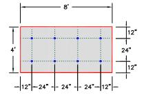
PERIMETER ZONE 8 FASTENERS PER 4'X8' BOARD
