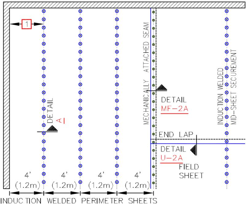
**PERIMETER SHEET SECUREMENT – FINGER METHOD**
