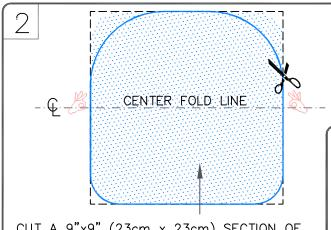
CUT A 9"x9" (23cm x 23cm) SECTION OF SURE-WHITE OR COOL GRAY PRESSURE-SENSITIVE UNCURED FLASHING AND MAKE ROUNDED CORNERS AS SHOWN.
