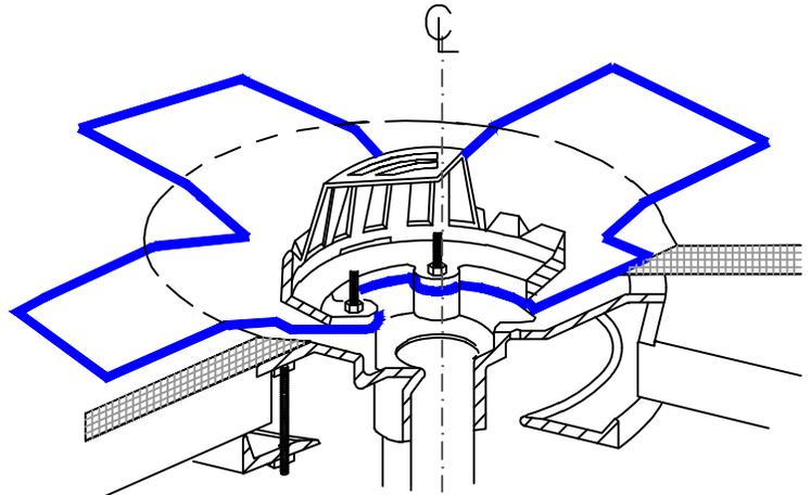
EXTEND TPO MEMBRANE ONTO MEMBRANE SECTION POSITIONED AT DRAIN SUMP AND CUT AS SHOWN TO LAY FLAT IN SUMP. HOT AIR WELD A MINIMUM OF 1-1/2" (4cm) COMPLETELY SURROUNDING AREA.
