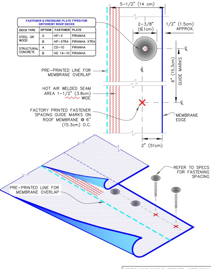
MECHANICALLY FASTENED ASSEMBLY
