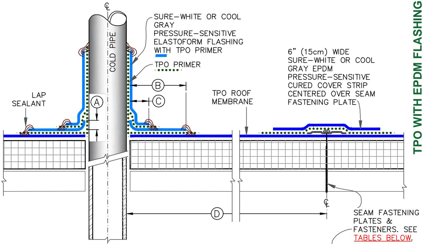
TPO WITH EPDM FLASHING
