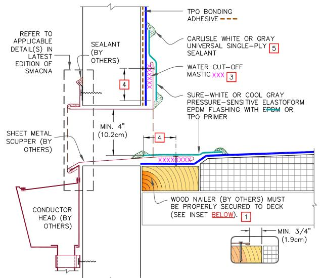
WOOD NAILERS ARE INSTALLED AT SCUPPERS TO SECURE METAL SLEEVE AND MUST EXTEND PAST THE WIDTH OF METAL SLEEVE FLANGE.
