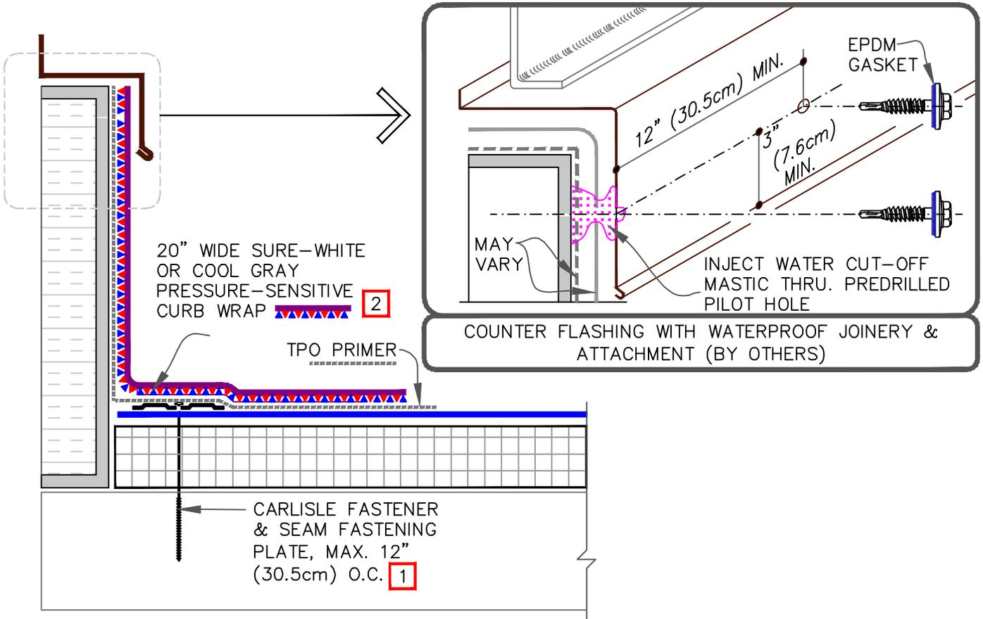
TPO WITH EPDM FLASHING
