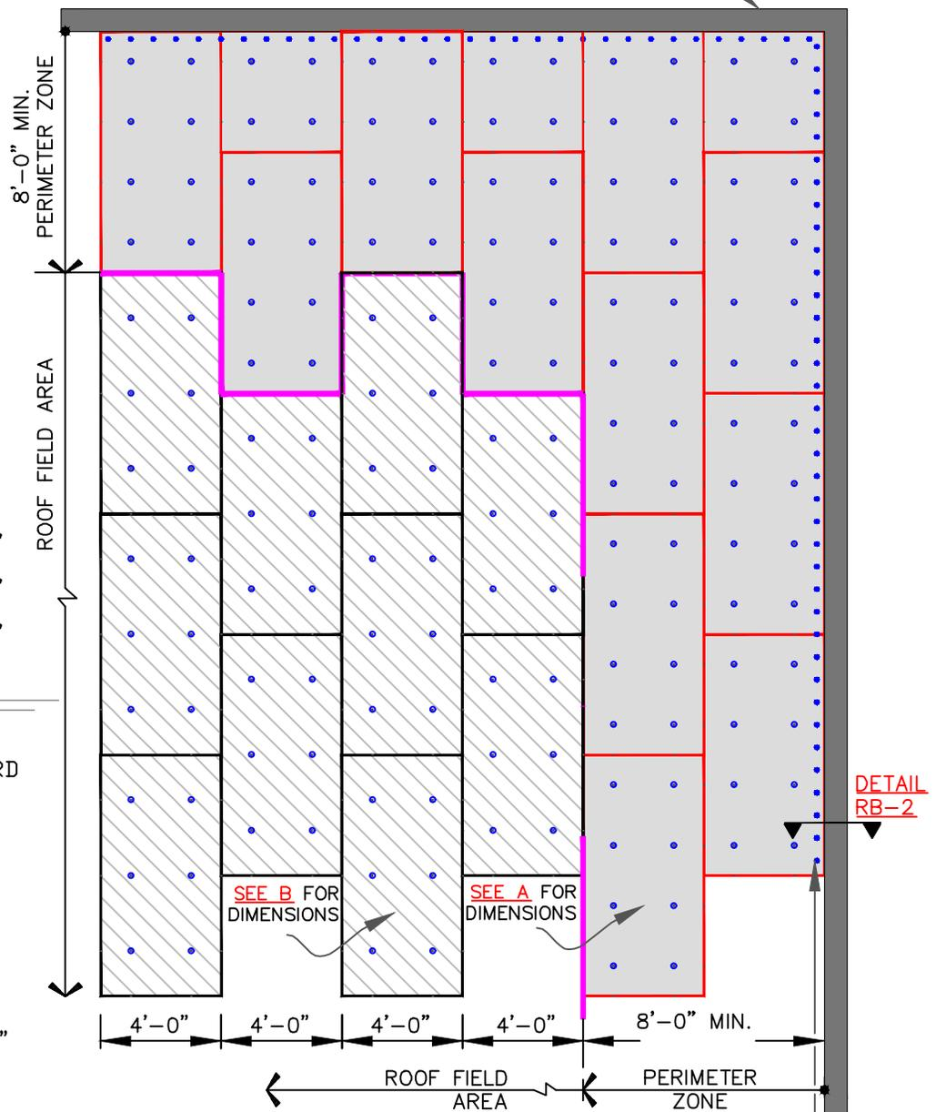
MEMBRANE FASTENED MINIMUM 12" O.C. AT ANGLE(S) CHANGES. FOR ADDITIONAL INFORMATION SEE DETAIL RB-2
