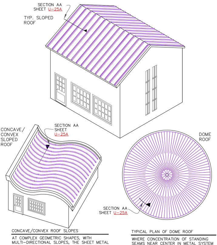
MULTI-DIRECTIONAL SLOPES, THE SHEET METAL ROOF IS NOT ONLY DIFFICULT TO INSTALL, BUT THE WATER-SHEDDING ABILITY OF METAL ROOF IS SERIOUSLY HAMPERED WITHIN THE CONCAVE (NEGATIVE) SLOPES. THE WATERPROOFED ROOF MEMBRANE WITH THE CONTOUR RIB IS A PRACTICAL SOLUTION.
