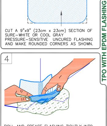
ROLL AND CREASE FLASHING TIGHTLY INTO ANGLE CHANGE AND FIRMLY ROLL FLASHING ONTO THE DECK MEMBRANE.
