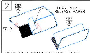
PRIOR TO PLACEMENT OF SURE-WHITE PRESSURE-SENSITIVE SURE-WHITE OR COOL GRAY CORNER, PEEL OFF THE POLY RELEASE FILM FROM THE FLASHING SIDE AND HEAT WITH A HEAT GUN. RE-APPLY THE POLY LOOSELY. FOLD THE FLASHING IN HALF.
