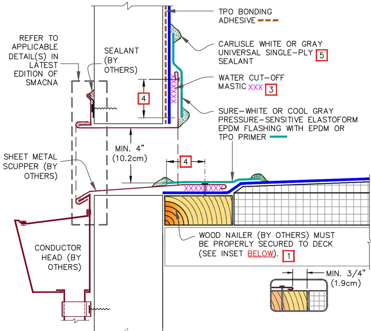
TPO WITH EPDM FLASHING
