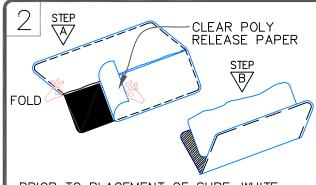
PRIOR TO PLACEMENT OF SURE-WHITE PRESSURE-SENSITIVE SURE-WHITE OR COOL GRAY CORNER, PEEL OFF THE POLY RELEASE FILM FROM THE FLASHING SIDE AND HEAT WITH A HEAT GUN. RE-APPLY THE POLY LOOSELY. FOLD THE FLASHING IN HALF.
