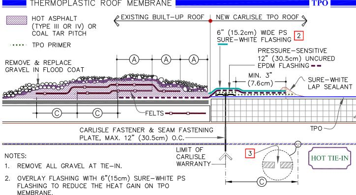
3. IF FLUTES ARE PERPENDICULAR TO THE TIE-IN DRILL A 3/8" (1cm) DIAMETER WEEP HOLE INTO THE BOTTOM FLUTES OF THE STEEL DECK ALONG THE PERIMETER OF THE TIE-IN 6" (15cm) MINIMUM TO 12" (30cm) MAXIMUM FROM THE SEAM FASTENING PLATE. HOLES MAY NOT BE REQUIRED IF DECK SLOPES DOWN TOWARDS EXISTING ROOF.
