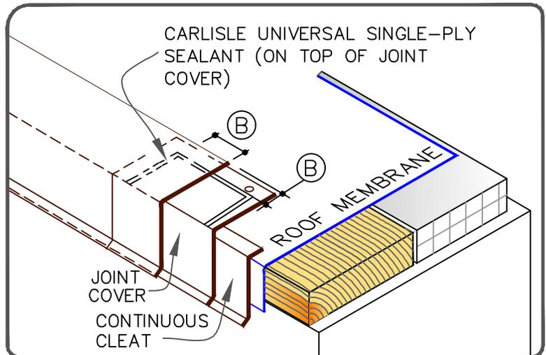
TPO WITH EPDM FLASHING
