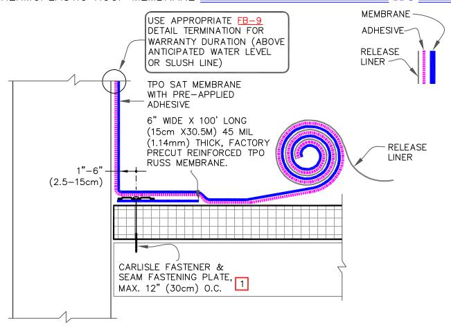
1. WIND SPEED GREATER THAN 90 MPH (145 KILOMETERS /HOURS)(40.3 METER PER SECOND) OR PROJECTS WITH 25 OR 30-YEAR WARRANTIES REQUIRE FASTENING @ 6"(15.2cm) 0.C.
