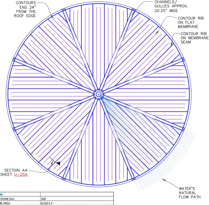
DOME TYP. DOME DIA DOME AREA **MEMBRANE** 81" ROLL WIDTH MEMBRANE SEAM WIDTH 2" WELDED PORTION CHANNELS/GULLIES PERFECTLY CUT 1/4TH WIDTH OF 81" ROLL (20.25") PERFECTLY CUT CIRCULAR SHAPE AS DESIGNED, APEX POINT APPRX. 37" DIA SHOWN **CONTOUR RIBS** CONTOUR RIBS O.C. 26.333" TOTAL LENGTH OF CONTOUR RIBS 3256 LINEAR FEET (ADD % FOR DOME CURVE) ON ENTIRE 100 DIA DOME
