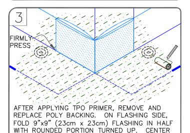
FLASHING ON CORNER AND FIRMLY PRESS
