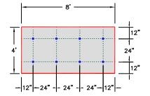
PERIMETER ZONE 8 FASTENERS PER 4'X8' BOARD
