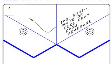
FASTEN MEMBRANE AND FLASH CURB OR WALL WITH MEMBRANE FOLLOWING STANDARD PROCEDURES USING BONDING ADHESIVE AND SURE-WHITE PRESSURE-SENSITIVE TAPE OR HOT AIR WELDING.
