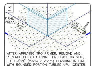
FLASHING ON CORNER AND FIRMLY PRESS
