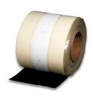
**TPO Pressure-Sensitive RUSS** 10" RUSS (shown) is used in place of narrow width sheets to secure membrane in the perimeter of the roof. 6" RUSS is used to secure membrane at the base of vertical walls without penetrating the sheet.
