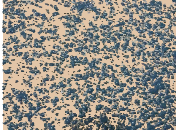
FIG 1. CORRECT COVERAGE – SPLATTER APPLICATION
