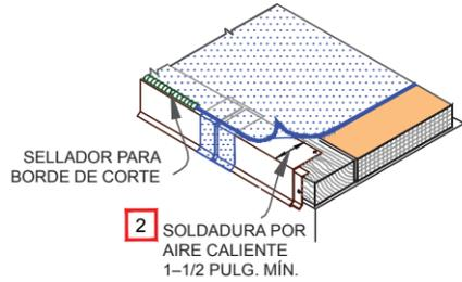
POSICIONE LA MEMBRANA DE CAMPO Y SUELDE POR CALOR EL METAL REVESTIDO COMO MÍNIMO EN 1-1/2 PULG. (38 mm), COMO MUESTRA LA FIGURA.
