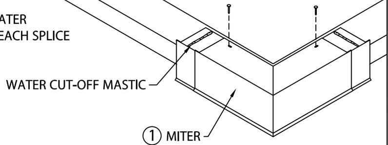
STEP ② POSITION 12'-0" CONTINUOUS CLEAT SECTIONS UNDER SPLICE PLATE AND MITER THEN FASTEN 12" O.C. AS SHOWN WITH PROVIDED FASTENERS. LAP CONTINUOUS CLEAT 1" AT JOINTS.
