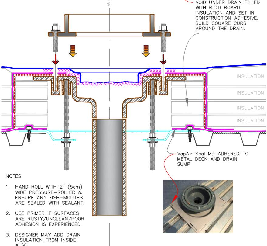
VapAir Seal MD ADHERED TO METAL DECK AND DRAIN SUMP
