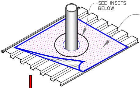
PROPERLY MARK A REQUIRED SIZE HOLE IN VapAir Seal MD AND CUT IT IN CIRCLE FOR ROUND PENETRATIONS AND FULLY ADHERE IT.
