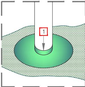
1 PRESSURE-SENSITIVE ELASTOFORM FLASHING IN CONJUNCTION WITH EPDM PRIMER.
