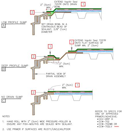
ADHESION IS EXPERIENCED. VapAir Seal MD ADHERED TO METAL DECK AND STEEL PLATE.
