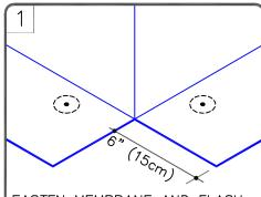
FASTEN MEMBRANE AND FLASH CURB OR WALL WITH CURED EPDM MEMBRANE FOLLOWING STANDARD PROCEDURES.
