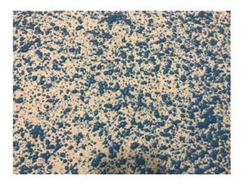
FIG 1. CORRECT COVERAGE - SPLATTER **APPLICATION**
