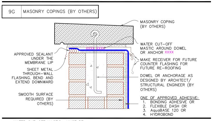
WATER CUT-OFF MASTIC- MUST BE HELD UNDER CONSTANT COMPRESSION.
