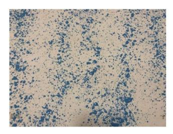
FIG 2. LIGHT COVERAGE - SPLATTER **APPLICATION**
