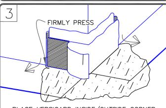
PLACE VERSIGARD INSIDE/OUTSIDE CORNER AS SHOWN AND REMOVE RELEASE PAPER. PRESS FOLDED FLASHING TIGHTLY INTO ANGLE CHANGE AND FIRMLY PRESS FLASHING AGAINST THE VERTICAL SURFACE.
