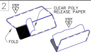
PRIOR TO PLACEMENT OF SURE—SEAL CORNER, PEEL OFF THE BLUE POLY RELEASE FILM AND HEAT THE FLASHING SIDE WITH A HEAT GUN. RE—APPLY THE POLY LOOSELY. FOLD THE FLASHING IN HALF.
