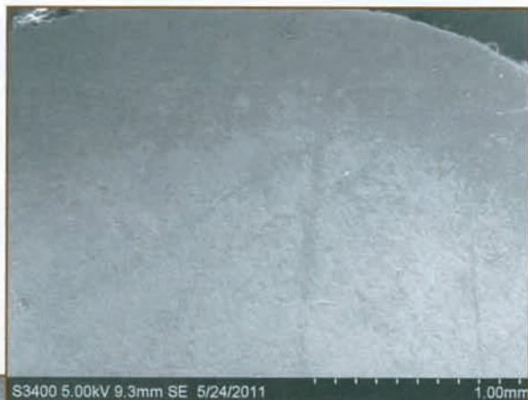
Figure 1 – 45-mil TPO at 50x magnification after 25,200 kJ-m 2 in a xenon arc weatherometer.
