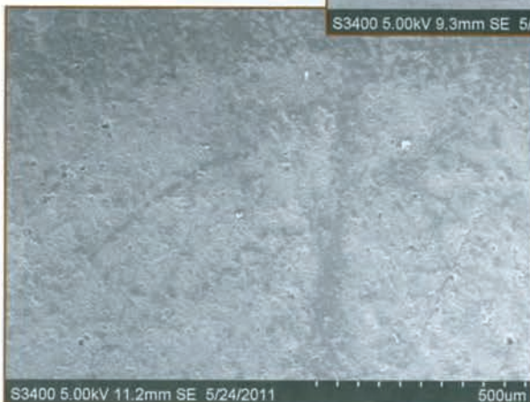
Figure 2 – 45-mil TPO at 100x magnification after 25,200 kJ-m 2 in a xenon arc weatherometer.
