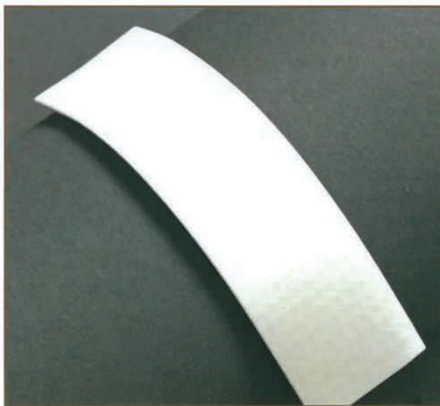
Figure 5 – Sample of TPO membrane exposed to 240°F for over 32 weeks.
