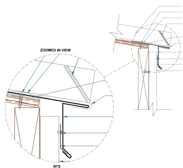
CM 200S PANEL #10 - 13 x 1" PHW (12" o.c.) CARLISLE 300 WIP UNDERLAYMENT CARLISLE APPROVED TUBE SEALANT (FIELD APPLIED BETWEEN PANEL RIBS)
