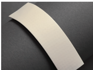
Carlisle Sure-Weld TPO – 60 Weeks (No Failure)
