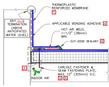
U-12A Parapet Flashing
