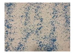
Fig 3. Correct Coverage – Splatter Application
