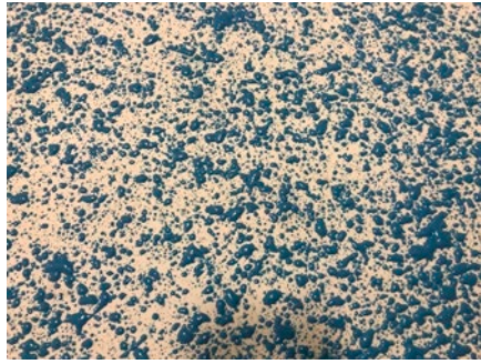
Fig 3. Correct Coverage – Splatter Application
