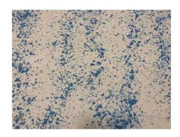
FIG 2. LIGHT COVERAGE - SPLATTER **APPLICATION**
