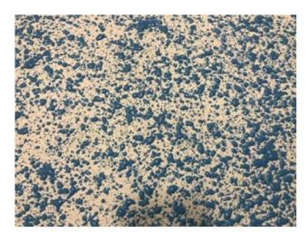
FIG 1. CORRECT COVERAGE - SPLATTER **APPLICATION**
