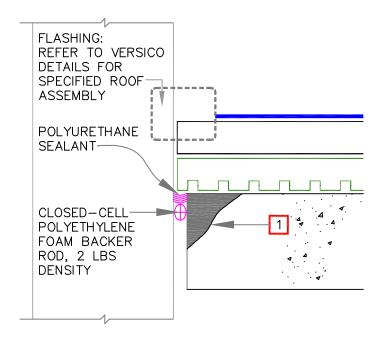
AIR SEAL: ROOF-TO-WALL
