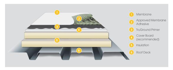
**Typical Roof Assembly with Conductive Primer**
