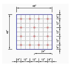
14 Insulation Fasteners & Plates
