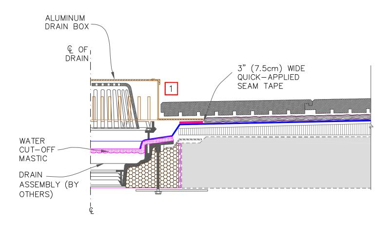
1. RUBBER PAVERS SHOULD BUTT TIGHTLY TO DRAIN BOXES TO MAINTAIN COMPRESSION.
