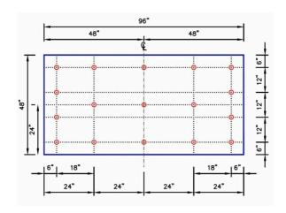
17 Insulation Fasteners & Plates
