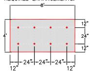
PERIMETER ZONE 8 FASTENERS PER 4'X8' BOARD
