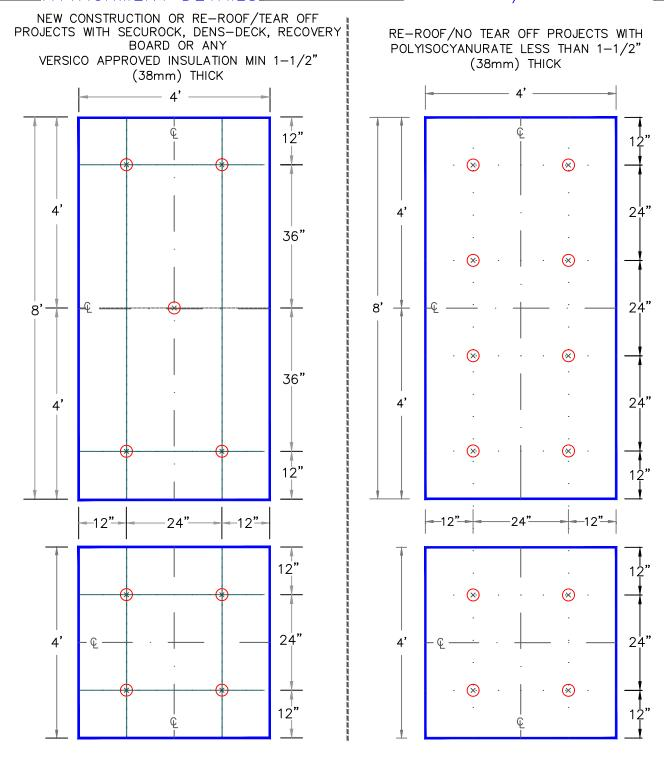
FOR CRITERIA ON INSULATION FASTENERS AND PLATES, REFER TO VERSICO SPECIFICATIONS.
