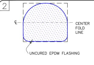
CUT A 9"x9" (23cm x 23cm) SECTION OF QUICK—APPLIED UNCURED EPDM FLASHING AND MAKE ROUNDED CORNERS AS SHOWN.
