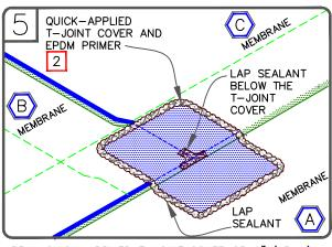
APPLY QUICK-APPLIED T-JOINT COVER OR 6" (15cm) WIDE SECTION OF QUICK-APPLIED UNCURED EPDM FLASHING CENTERED OVER THE INTERSECTING POINT OF THE LEADING EDGES OF THE FIELD SPLICE INTERSECTION AS SHOWN.
