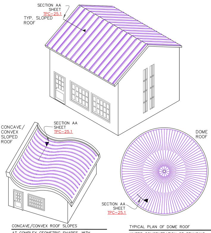
AT COMPLEX GEOMETRIC SHAPES, WITH MULTI-DIRECTIONAL SLOPES, THE SHEET METAL ROOF IS NOT ONLY DIFFICULT TO INSTALL, BUT THE WATER-SHEDDING ABILITY OF METAL ROOF IS SERIOUSLY HAMPERED WITHIN THE CONCAVE (NEGATIVE) SLOPES. THE WATERPROOFED ROOF MEMBRANÉ WITH THE CONTOUR RIB IS A PRACTICAL SOLUTION.
