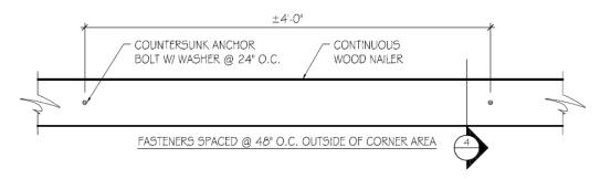
FIGURE 7B - TYPICAL ROOF EDGE WOOD BLOCKING - THROUGH BOLT ANCHORAGE
