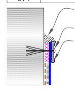
VERSICO UNIVERSAL SINGLE-PLY SEALANT OR SEALANT (BY OTHERS) VERSICO ZINC NAIL-IN ANCHOR
