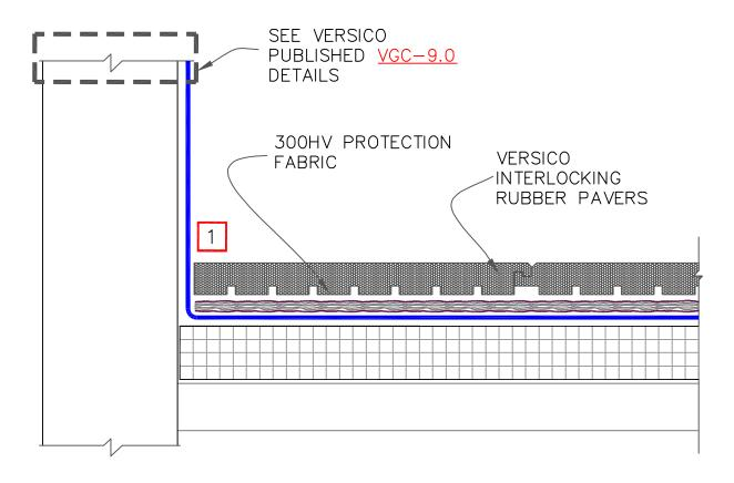
1. RUBBER PAVERS SHOULD BUTT TIGHTLY TO PARAPET WALLS. REFER TO VERSICO'S RUBBER PAVER INSTALLATION GUIDE FOR MORE INFORMATION.
