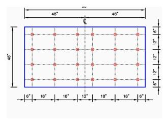
24 Insulation Fasteners & Plates
