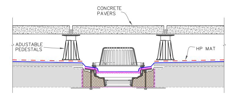
1. THIS OPTION IS ONLY APPLICABLE TO PAVERS ON ADJUSTABLE PEDESTALS WHEN THERE IS ENOUGH HEIGHT ADJUSTMENT TO CLEAR DRAIN BASKETS
