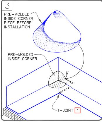
1. WHEN USING 60 OR 80-MIL MEMBRANE, APPLY A 4-1/2" (11cm) DIAMETER "T-JOINT" COVER AT ALL FIELD SPLICE INTERSECTIONS.
