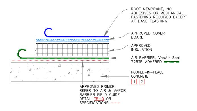
THE SUBSTRATE MAY NOT REQUIRE AN ADDITIONAL LAYER OF AIR BARRIER. TO ENSURE THAT A CONTINUOUS AIR-SEAL IS PROVIDED, THE SUBSTRATE MUST BE INSPECTED FOR BREACHES FOR AIR INFILTRATION AT CRACKS, JOINTS, PENETRATIONS, ROOF EDGES, PARAPET WALLS, AND SIMILAR CONDITIONS.
