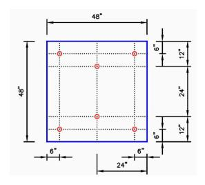
6 Insulation Fasteners & Plates
