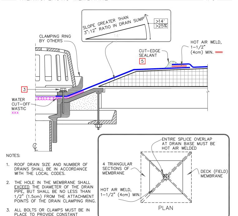
4. REMOVE EXISTING LEAD, FLASHING MATERIAL & ENSURE THE DRAIN RING IS COMPLETELY CLEAN DOWN TO BARE METAL.
