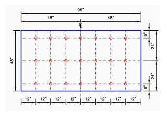
21 Insulation Fasteners & Plates
