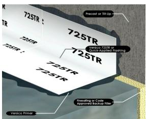
Gaps must be filled with firesafing or building code approved backup filler.
