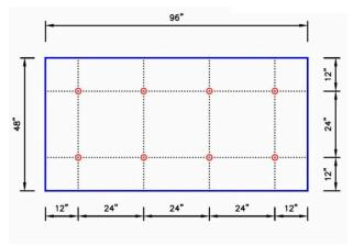
8 Insulation Fasteners & Plates
