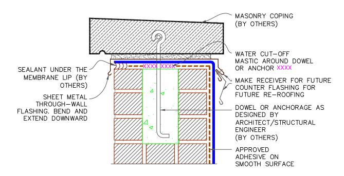
MAXIMUM WARRANTY: 30 YEARS WATER CUT-OFF MASTIC- MUST BE APPLICABLE BONDING ADHESIVE HELD UNDER CONSTANT COMPRESSION. ■ EPDM MEMBRANE **THERMOSET** ROOFING SYSTEM MEMBRANE TERMINATIONS → APPROVED SUBSTRATE (PAGE 3 OF 3) -9.00 ROOFING SYSTEMS 0 → SEE NOTE(S) MAXIMUM WARRANTY: 30 YEARS © 2024 VERSICO
