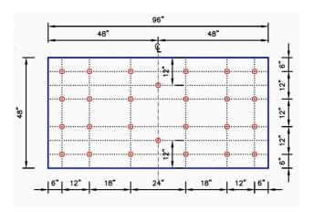
26 Insulation Fasteners & Plates
