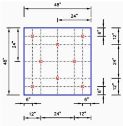
8 Insulation Fasteners & Plates
