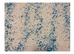
Fig 3. Correct Coverage - Splatter Application
