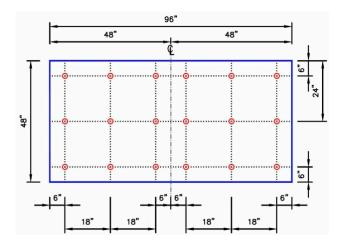
18 Insulation Fasteners & Plates
