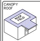
INSTALL PERIMETER SHEETS OVER THE ENTIRE OVERHANG (PROJECTION ROOF) AREA, EXTENDING ONTO THE MAIN ROOF DECK WHEN AT THE SAME LEVEL AS SHOWN.
