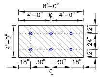
FIELD OF ROOF 6 FASTENERS PER 4'X8' BOARD
