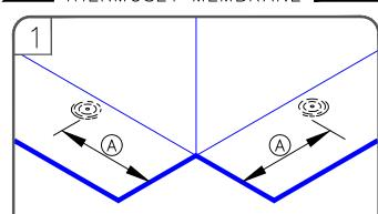
FASTEN MEMBRANE AND FLASH CURB OR WALL WITH CURED EPDM MEMBRANE FOLLOWING STANDARD PROCEDURES USING BONDING ADHESIVE and QA SEAM TAPE.
