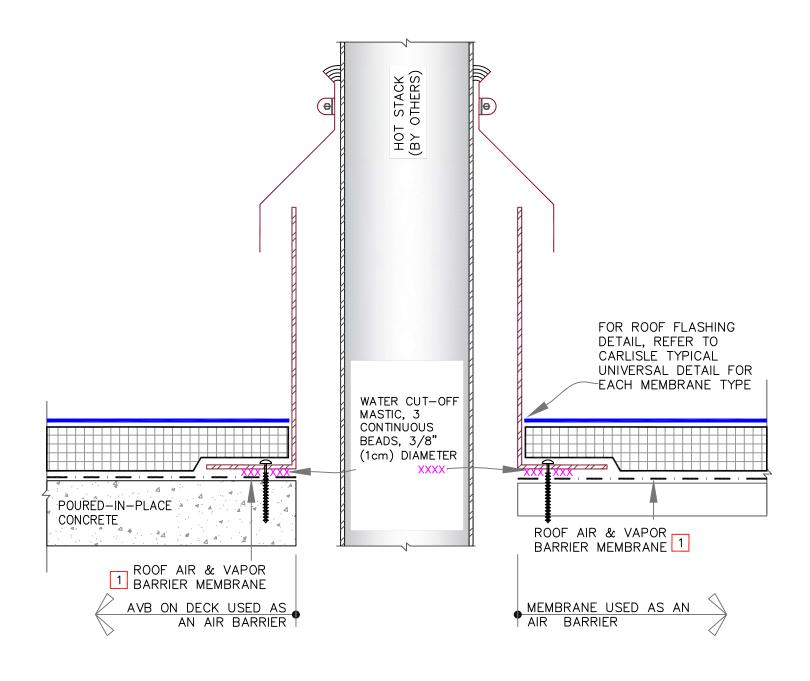
ON STEEL DECKS DIRECTLY ADHERE VapAir Seal MD. USE VapAir Seal 725TR ON CONCRETE & WOOD DECKS OR DECKS WITH APPROVED COVER BOARDS.
