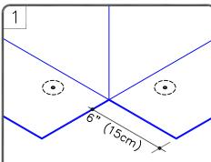
FASTEN MEMBRANE AND FLASH CURB OR WALL WITH CURED EPDM MEMBRANE FOLLOWING STANDARD PROCEDURES.
