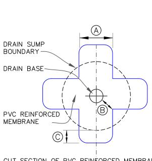
EXTEND PVC MEMBRANE ONTO MEMBRANE SECTION POSITIONED AT DRAIN SUMP AND CUT AS SHOWN TO LAY FLAT IN SUMP. HOT AIR WELD A MINIMUM OF 1-1/2" (4cm) COMPLETELY SURROUNDING AREA.
