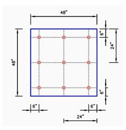
9 Insulation Fasteners & Plates
