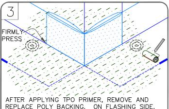
REPLACE POLY BACKING. ON FLASHING SIDE, FOLD 9"x9" (23cm x 23cm) FLASHING IN HALF WITH ROUNDED PORTION TURNED UP. CENTER FLASHING ON CORNER AND FIRMLY PRESS AGAINST VERTICAL SURFACE.
