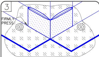
AFTER APPLYING EPDM PRIMER, REMOVE AND REPLACE POLY BACKING. FOLD FLASHING IN HALF WITH ROUNDED PORTION TURNED UP. CENTER FLASHING ON CORNER AND FIRMLY PRESS AGAINST VERTICAL SURFACE.
