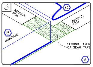
SPLICE SHEET B TO SHEET A AND APPLY SECOND PIECE OF QA SEAM TAPE BETWEEN SHEET B AND C. TRIM RELEASE FILM AS SHOWN.
