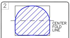
USE PRE-CUT T-JOINT COVERS OR CUT A 6"x6" (15X15cm) & 12"x12" (30X30cm) SECTION OF QUICK-APPLIED UNCURED FLASHING AND ROUND CORNERS
