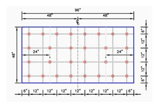
28 Insulation Fasteners & Plates
