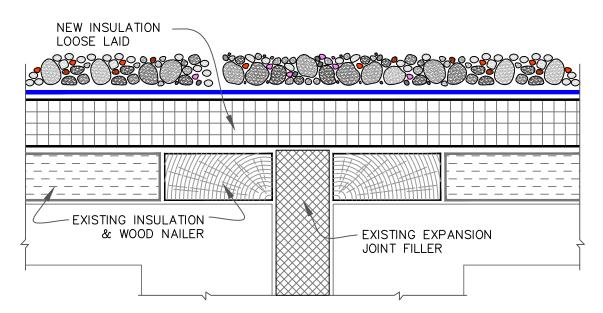
REROOFING OR RECOVER OF EXISTING ROOF
