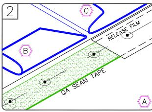
FOLD SHEETS BACK AS SHOWN. APPLY EPDM PRIMER TO THE SPLICE AREA ON BOTH SURFACES AND ALLOW TO FLASH-OFF. APPLY QA SEAM TAPE WITH RELEASE FILM ALIGNED WITH PRE-MARKED LINE.
