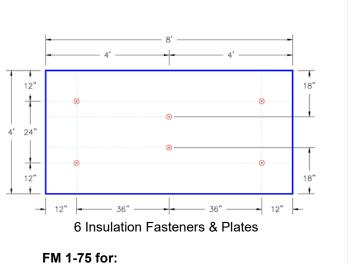
1/2" Securock (with InsulTite fasteners and SecurFAST Plates)
