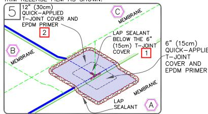
APPLY 6" (15cm) QUICK-APPLIED T-JOINT COVER AND 12" (30cm) QUICK-APPLIED T-JOINT COVER OR QUICK-APPLIED UNCURED CENTERED OVER THE INTERSECTING POINT OF THE LEADING EDGES OF THE FIELD SPLICE INTERSECTION AS SHOWN.
