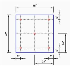
5 Insulation Fasteners & Plates
