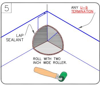
TPO PRIMER MUST BE APPLIED TO ALL SPLICE AREAS AND FOR EACH LAYER OF PEEL & STICK FLASHING.
