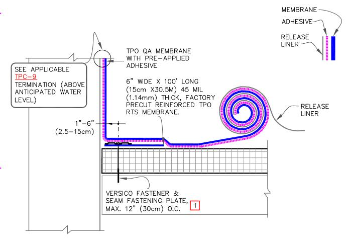
1. WIND SPEED GREATER THAN 90 MPH (145 KILOMETERS /HOURS)(40.3 METER PER SECOND) OR PROJECTS WITH 25 OR 30-YEAR WARRANTIES REQUIRE FASTENING @ 6"(15.2cm) O.C.
