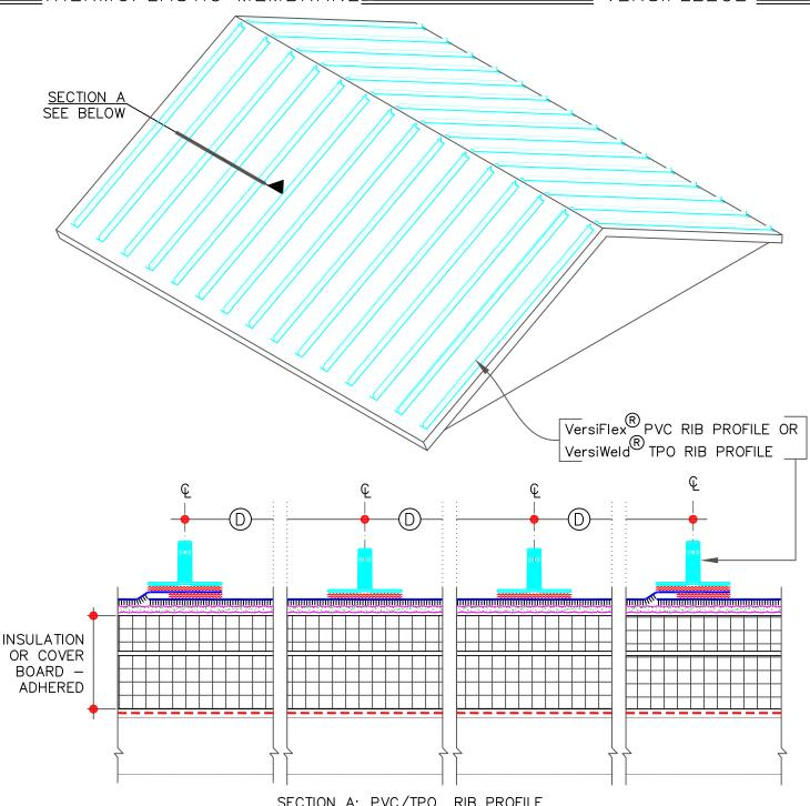
SECTION A: PVC/TPO RIB PROFILE
