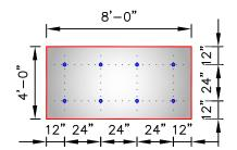
PERIMETER ZONE 8 FASTENERS PER 4'X8' BOARD
