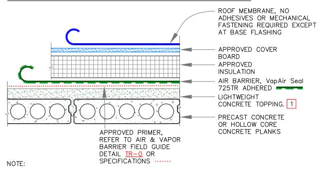
THE SUBSTRATE MAY NOT REQUIRE AN ADDITIONAL LAYER OF AIR BARRIER WHEN CONCRETE TOPPING EXISTS. TO ENSURE THAT A CONTINUOUS AIR-SEAL IS PROVIDED, THE SUBSTRATE MUST BE INSPECTED FOR BREACHES FOR AIR INFILTRATION AT CRACKS, JOINTS, PENETRATIONS, ROOF EDGES, PARAPET WALLS, AND SIMILAR CONDITIONS & PROPER REPAIRS MUST BE PERFORMED.
