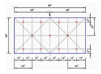
11 Insulation Fasteners & Plates
