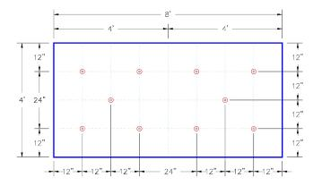
10 Insulation Fasteners & Plates
