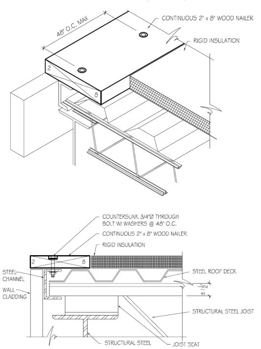
FIGURE 4 - ROOF EDGE WOOD BLOCKING - THROUGH BOLT ANCHORS
