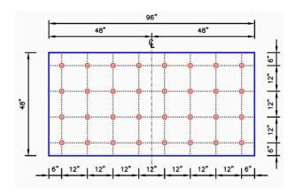
32 Insulation Fasteners & Plates
