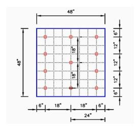
11 Insulation Fasteners & Plates
