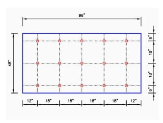
15 Insulation Fasteners & Plates
