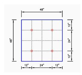
4 Insulation Fasteners & Plates
