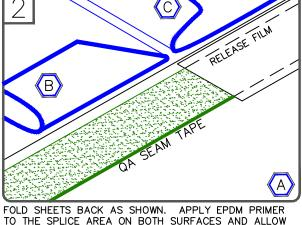
FOLD SHEETS BACK AS SHOWN. APPLY EPDM PRIMER TO THE SPLICE AREA ON BOTH SURFACES AND ALLOW TO FLASH-OFF. APPLY QA SEAM TAPE WITH RELEASE FILM ALIGNED WITH MARKED LINE.
