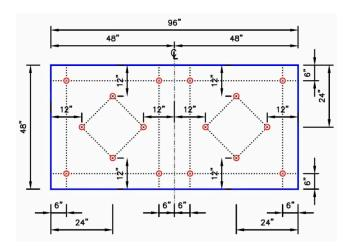
16 Insulation Fasteners & Plates
