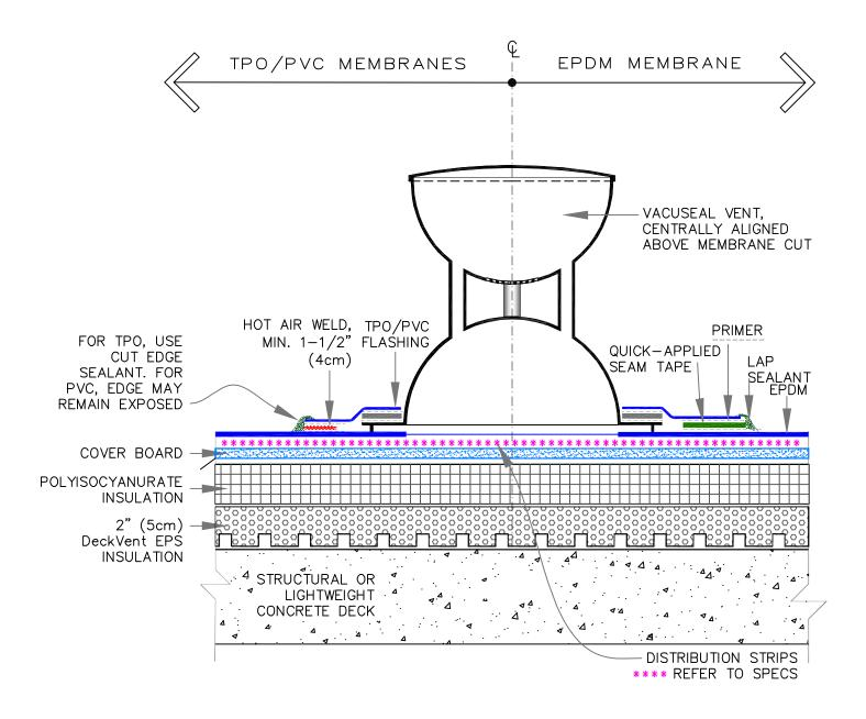
TOTAL NUMBER OF VENTS AND LOCATIONS ON THE ROOF WILL BE DETERMINED BY VERSICO. SUBMIT A COPY OF ROOF PLAN IN CAD TO VERSICO TO LOCATE VENTS. DESIGNER MUST SHOW ALL PENETRATIONS, HVAC UNITS, HEIGHT OF PARAPET WALLS AND HEIGHT OF ROOF FROM GROUND.
