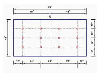
12 Insulation Fasteners & Plates
