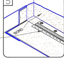
CUT 45° AND APPLY EPDM . PRIMER/QA SEAM TAPE
