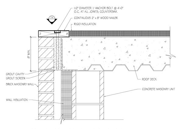
FIGURE 1 - ROOF EDGE WOOD BLOCKING - ANCHOR BOLT SECUREMENT
