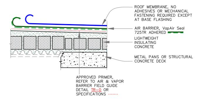
1. THE SUBSTRATE MAY NOT REQUIRE AN ADDITIONAL LAYER OF AIR BARRIER WHEN CONCRETE TOPPING EXISTS. TO ENSURE THAT CONCRETE SUBSTRATE PROVIDES A CONTINUOUS AIR—SEAL, THE SUBSTRATE MUST BE INSPECTED FOR AIR INFILTRATION. INSPECT FOR BREACHES CRACKS, JOINTS, PENETRATIONS, ROOF EDGES, PARAPET WALLS JUNCTIONS, AND SIMILAR CONDITIONS. PROPER REPAIRS MUST BE PERFORMED TO CREATE AN AIR BARRIER.
