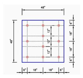
10 Insulation Fasteners & Plates
