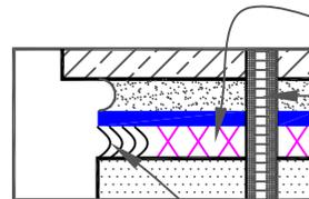
WATER CUT-OFF MASTIC AROUND DOWEL OR ANCHOR
