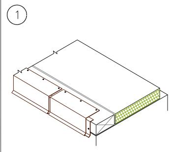
INSTALL CONTINUOUS CLEAT AND COATED METAL WITH 1/8"-1/4" (0.5cm-1cm) JOINTS BETWEEN ADJOINING SECTIONS.
