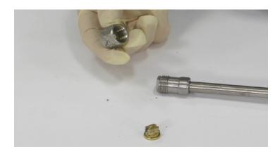
**Step 3:** Place a new spray tip or cleaned spray tip into the retaining cap. Turn the retaining cap onto the threaded extension assembly.
