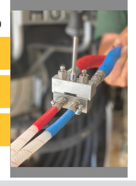
Tighten pump packing.
