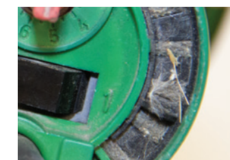
DIRT AND DEBRIS IN INTAKE
