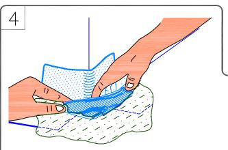
ROLL AND CREASE FLASHING TIGHTLY INTO ANGLE CHANGE AND FIRMLY ROLL FLASHING ONTO THE DECK MEMBRANE.
