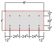
PERIMETER ZONE 8 FASTENERS PER 4'X8' BOARD
