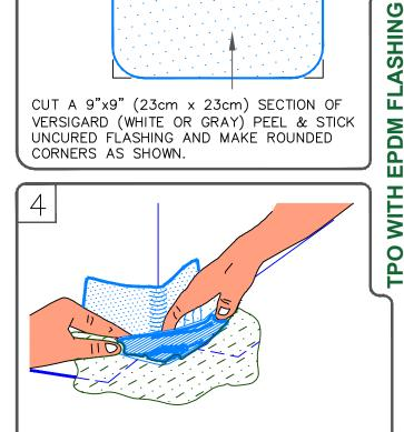
ROLL AND CREASE FLASHING TIGHTLY INTO ANGLE CHANGE AND FIRMLY ROLL FLASHING ONTO THE DECK MEMBRANE.
