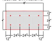
PERIMETER ZONE 8 FASTENERS PER 4'X8' BOARD
