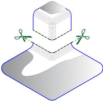
60-MIL (1.52mm) THICK TPO, UNIVERSAL CORNER CAN BE USED FOR AT TOP CORNER. CUT AS SHOWN IN DETAIL [TPC-15.7](#)
