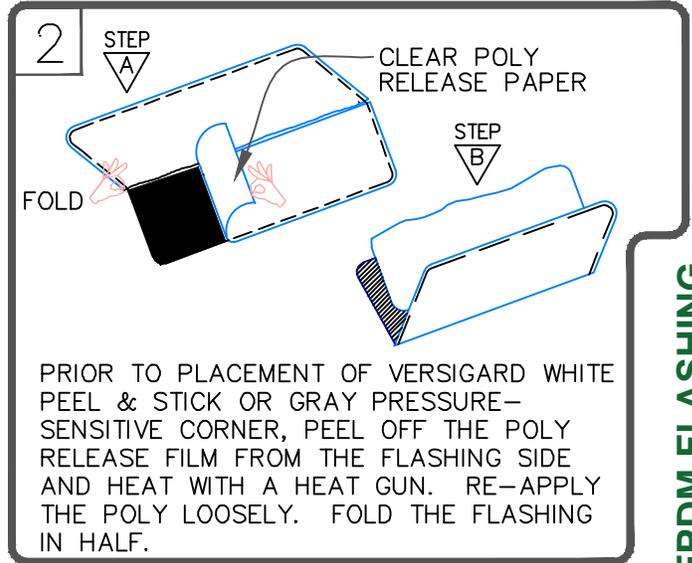
PRIOR TO PLACEMENT OF VERSIGARD WHITE PEEL & STICK OR GRAY PRESSURE-SENSITIVE CORNER, PEEL OFF THE POLY RELEASE FILM FROM THE FLASHING SIDE AND HEAT WITH A HEAT GUN. RE-APPLY THE POLY LOOSELY. FOLD THE FLASHING IN HALF.
