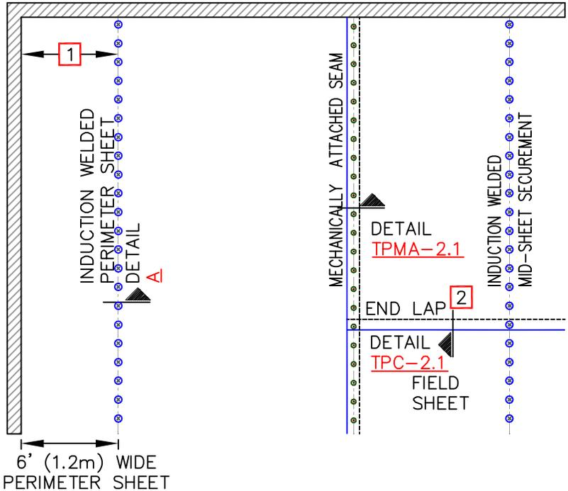
VERSICO FASTENER AND INDUCTION WELDING FASTENING PLATE, 12" (30cm) O.C. MAX.
