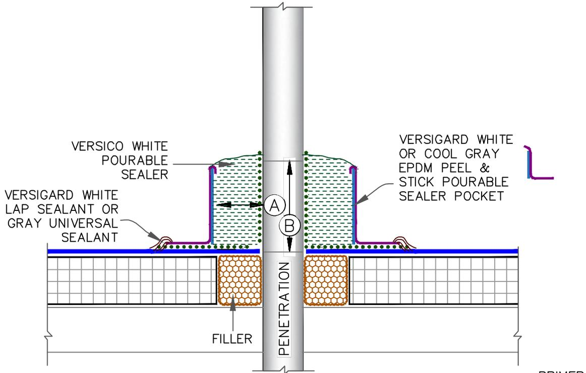
TPO WITH EPDM FLASHING
