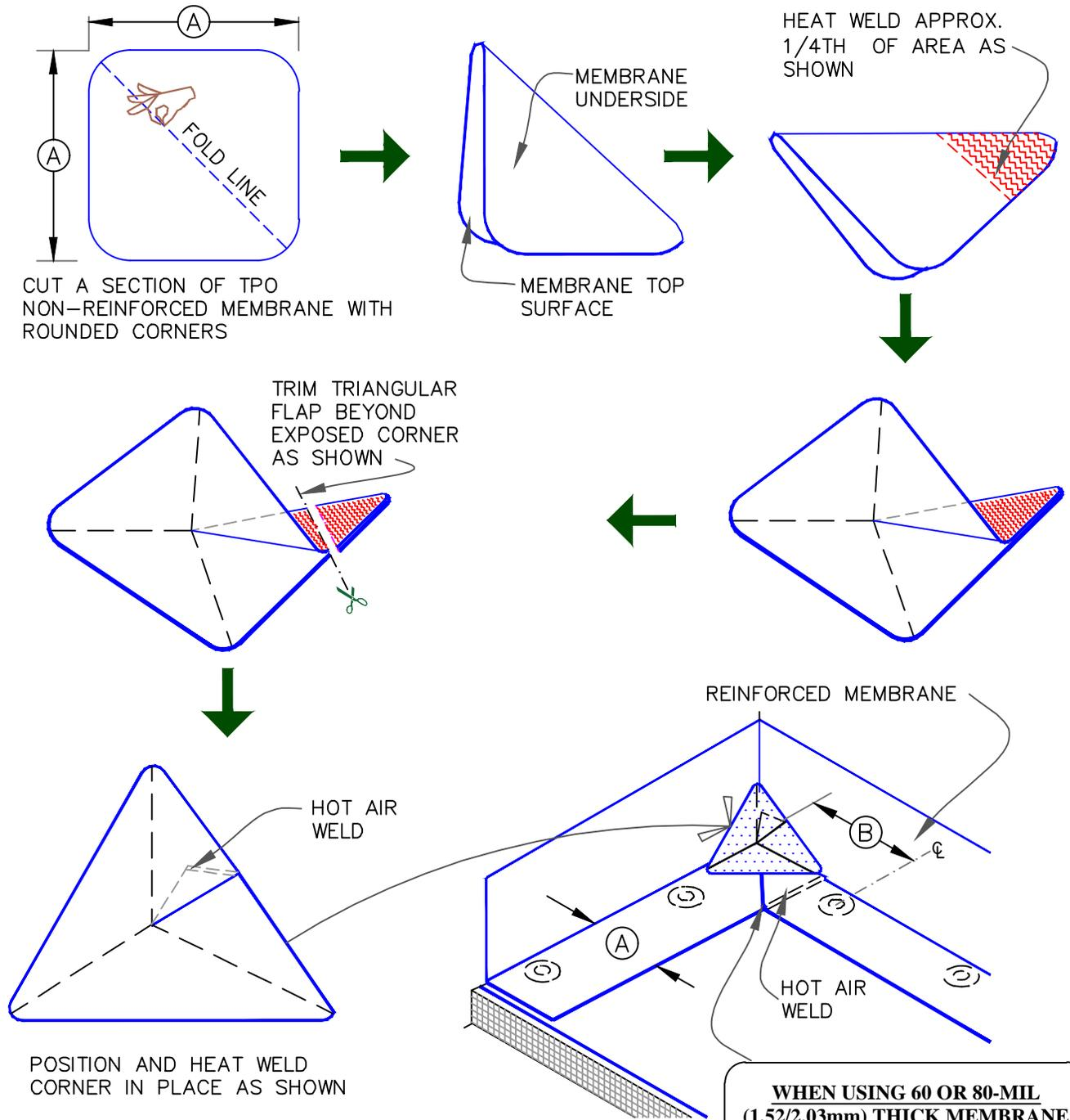
**WHEN USING 60 OR 80-MIL (1.52/2.03mm) THICK MEMBRANE**
