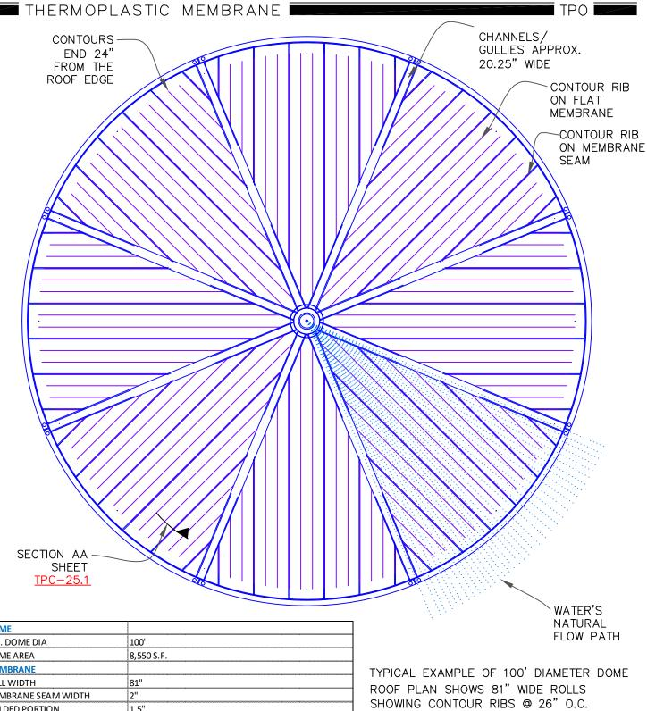
DOME TYP. DOME DIA DOME AREA **MEMBRANE** ROLL WIDTH MEMBRANE SEAM WIDTH WELDED PORTION CHANNELS/GULLIES PERFECTLY CUT 1/4TH WIDTH OF 81" ROLL (20.25") PERFECTLY CUT CIRCULAR SHAPE AS DESIGNED, APEX POINT APPRX. 37" DIA SHOWN **CONTOUR RIBS** CONTOUR RIBS O.C. 26.333" TOTAL LENGTH OF CONTOUR RIBS 3256 LINEAR FEET (ADD % FOR DOME CURVE) ON ENTIRE 100 DIA DOME
