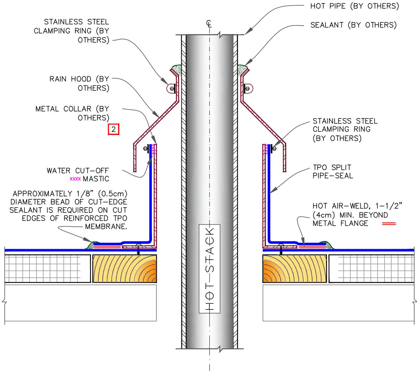
APPROXIMATELY 1/8" (0.5cm) DIAMETER BEAD OF CUT-EDGE SEALANT IS REQUIRED ON CUT EDGES OF REINFORCED TPO MEMBRANE.
