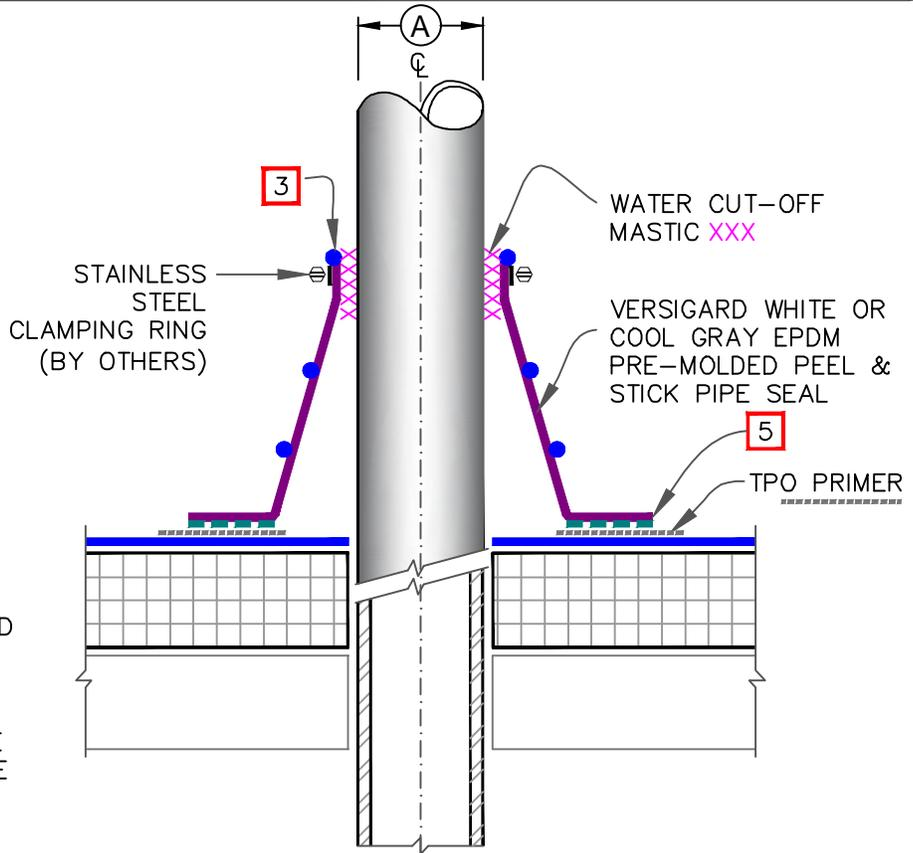
TPO WITH EPDM FLASHING
