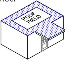
INSTALL PERIMETER SHEETS OVER THE ENTIRE OVERHANG (PROJECTION ROOF) AREA, EXTENDING ONTO THE MAIN ROOF DECK WHEN AT THE SAME LEVEL AS SHOWN.
