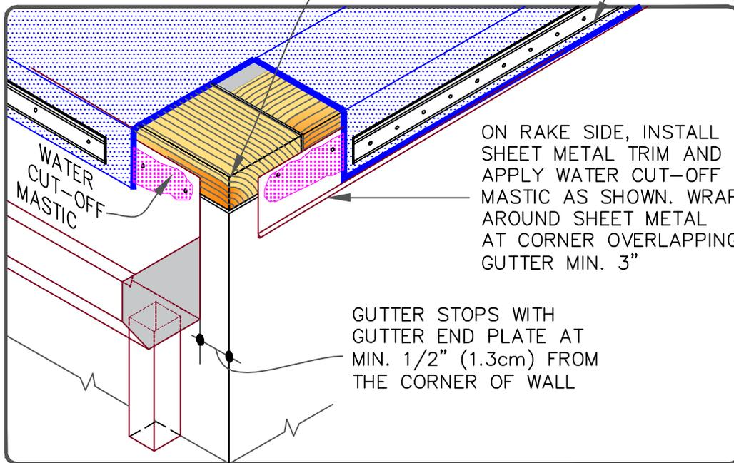
ON RAKE SIDE, INSTALL SHEET METAL TRIM AND APPLY WATER CUT-OFF MASTIC AS SHOWN. WRAP AROUND SHEET METAL AT CORNER OVERLAPPING GUTTER MIN. 3"
