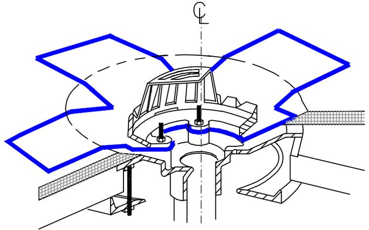
EXTEND TPO MEMBRANE ONTO MEMBRANE SECTION POSITIONED AT DRAIN SUMP AND CUT AS SHOWN TO LAY FLAT IN SUMP. HOT AIR WELD A MINIMUM OF 1-1/2" (4cm) COMPLETELY SURROUNDING AREA.
