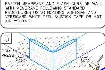
AFTER APPLYING TPO PRIMER, REMOVE AND REPLACE POLY BACKING. ON FLASHING SIDE, FOLD 9"x9" (23cm x 23cm) FLASHING IN HALF WITH ROUNDED PORTION TURNED UP. CENTER FLASHING ON CORNER AND FIRMLY PRESS AGAINST VERTICAL SURFACE.
