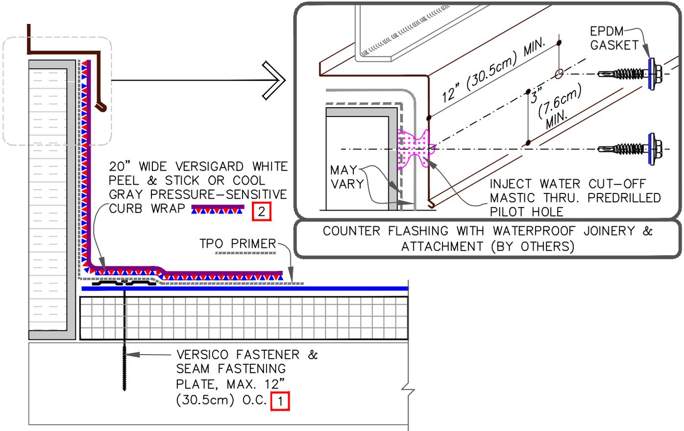
TPO WITH EPDM FLASHING
