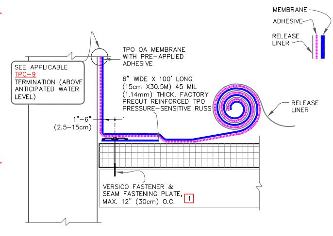
WIND SPEED GREATER THAN 90 MPH (145 KILOMETERS /HOURS)(40.3 METER PER SECOND) OR PROJECTS WITH 25 OR 30-YEAR WARRANTIES REQUIRE FASTENING @ 6"(15.2cm) 0.C.
