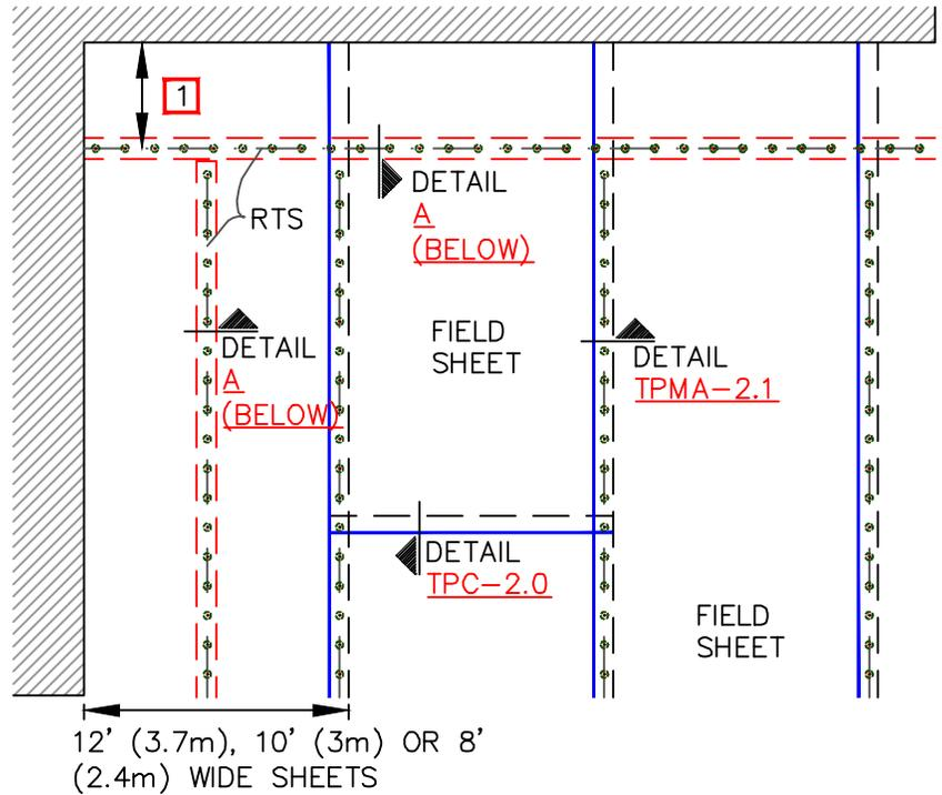
TPO PRIMER MUST BE APPLIED TO THE BACK SIDE OF MEMBRANE SURFACE PRIOR TO ADHERING MEMBRANE TO QA RTS.
