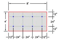
PERIMETER ZONE 8 FASTENERS PER 4'X8' BOARD
