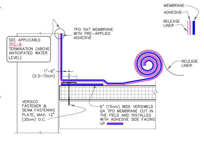
WIND SPEED GREATER THAN 90 MPH (145 KILOMETERS /HOURS)(40.3 METER PER SECOND) OR PROJECTS WITH 25 OR 30-YEAR WARRANTIES REQUIRE FASTENING @ 6"(15.2cm) O.C.
