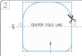
CUT A 9"x9" (23cm x 23cm) SECTION OF VERSIGARD (WHITE OR GRAY) PEEL & STICK UNCURED FLASHING AND MAKE ROUNDED CORNERS AS SHOWN.
