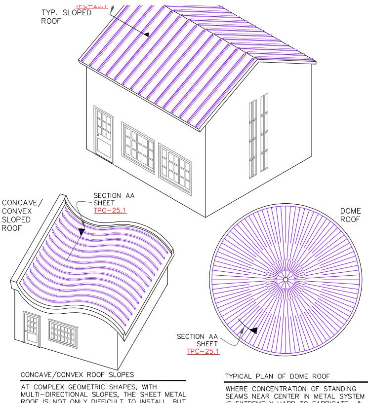
ROOF IS NOT ONLY DIFFICULT TO INSTALL, BUT THE WATER-SHEDDING ABILITY OF METAL ROOF IS SERIOUSLY HAMPERED WITHIN THE CONCAVE (NEGATIVE) SLOPES. THE WATERPROOFED ROOF MEMBRANE WITH THE CONTOUR RIB IS A PRACTICAL SOLUTION.
