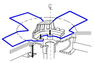
EXTEND TPO MEMBRANE ONTO MEMBRANE SECTION POSITIONED AT DRAIN SUMP AND CUT AS SHOWN TO LAY FLAT IN SUMP. HOT AIR WELD A MINIMUM OF 1-1/2" (4cm) COMPLETELY SURROUNDING AREA.
