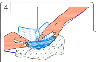
ROLL AND CREASE FLASHING TIGHTLY INTO ANGLE CHANGE AND FIRMLY ROLL FLASHING ONTO THE DECK MEMBRANE.
