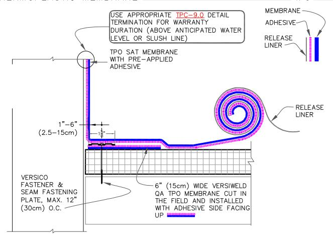
WIND SPEED GREATER THAN 90 MPH (145 KILOMETERS /HOURS)(40.3 METER PER SECOND) OR PROJECTS WITH 25 OR 30-YEAR WARRANTIES REQUIRE FASTENING @ 6"(15.2cm) O.C.
