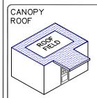
INSTALL PERIMETER SHEETS OVER THE ENTIRE OVERHANG (PROJECTION ROOF) AREA, EXTENDING ONTO THE MAIN ROOF DECK WHEN AT THE SAME LEVEL AS SHOWN.
