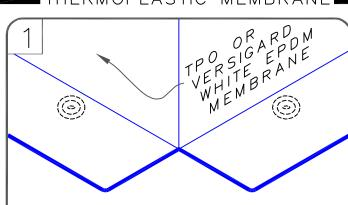
FASTEN MEMBRANE AND FLASH CURB OR WALL WITH MEMBRANE FOLLOWING STANDARD PROCEDURES USING BONDING ADHESIVE AND VERSIGARD WHITE PEEL & STICK TAPE OR HOT AIR WELDING.
