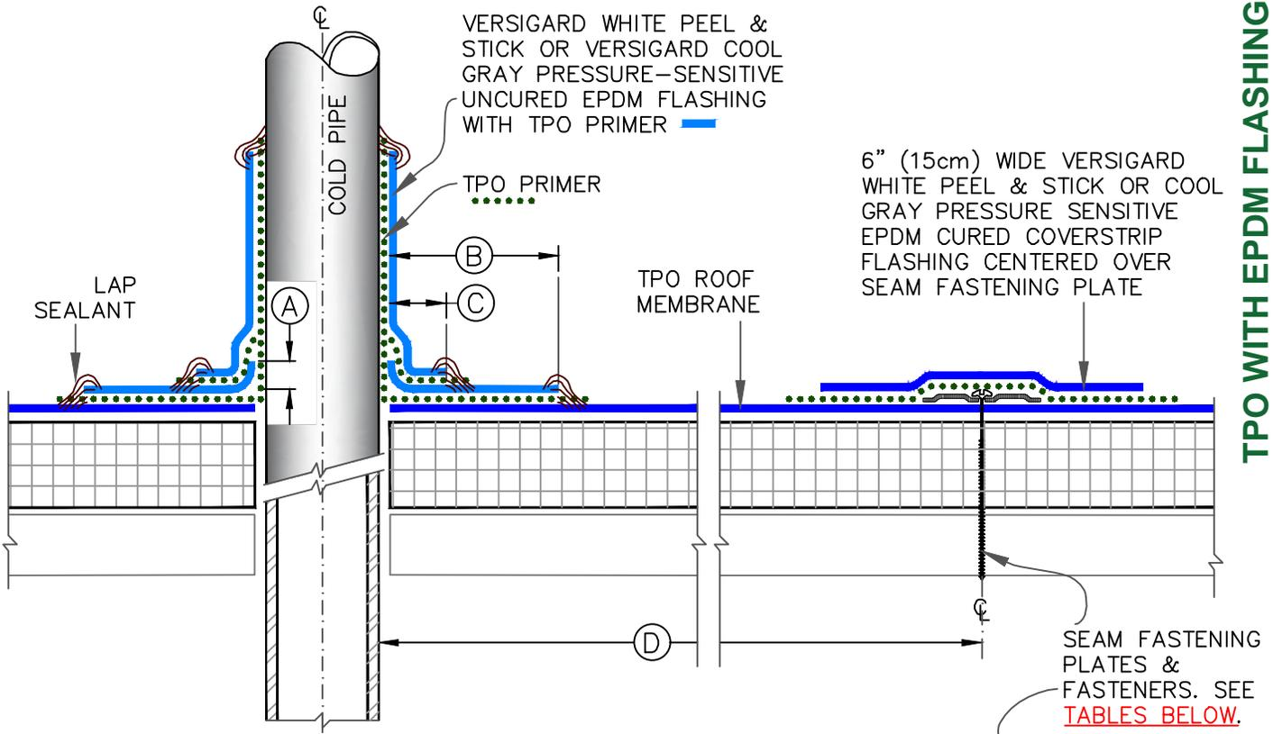
TPO WITH EPDM FLASHING
