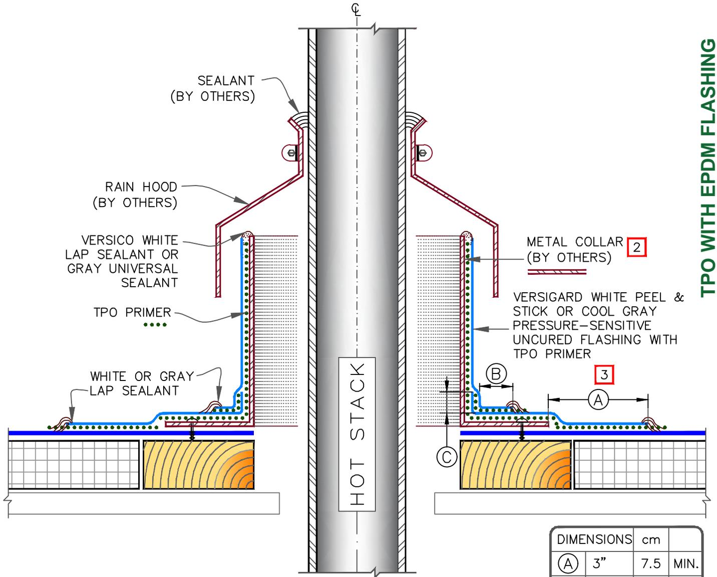
TPO WITH EPDM FLASHING
