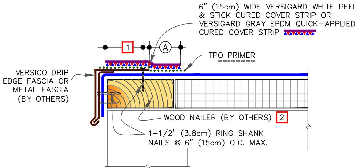
TPO WITH EPDM FLASHING
