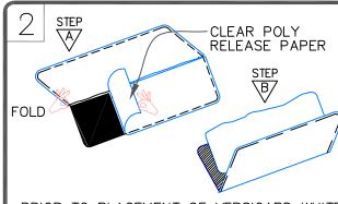
PRIOR TO PLACEMENT OF VERSIGARD WHITE PEEL & STICK OR GRAY PRESSURE-SENSITIVE CORNER, PEEL OFF THE POLY RELEASE FILM FROM THE FLASHING SIDE AND HEAT WITH A HEAT GUN. RE-APPLY THE POLY LOOSELY. FOLD THE FLASHING IN HALF.
