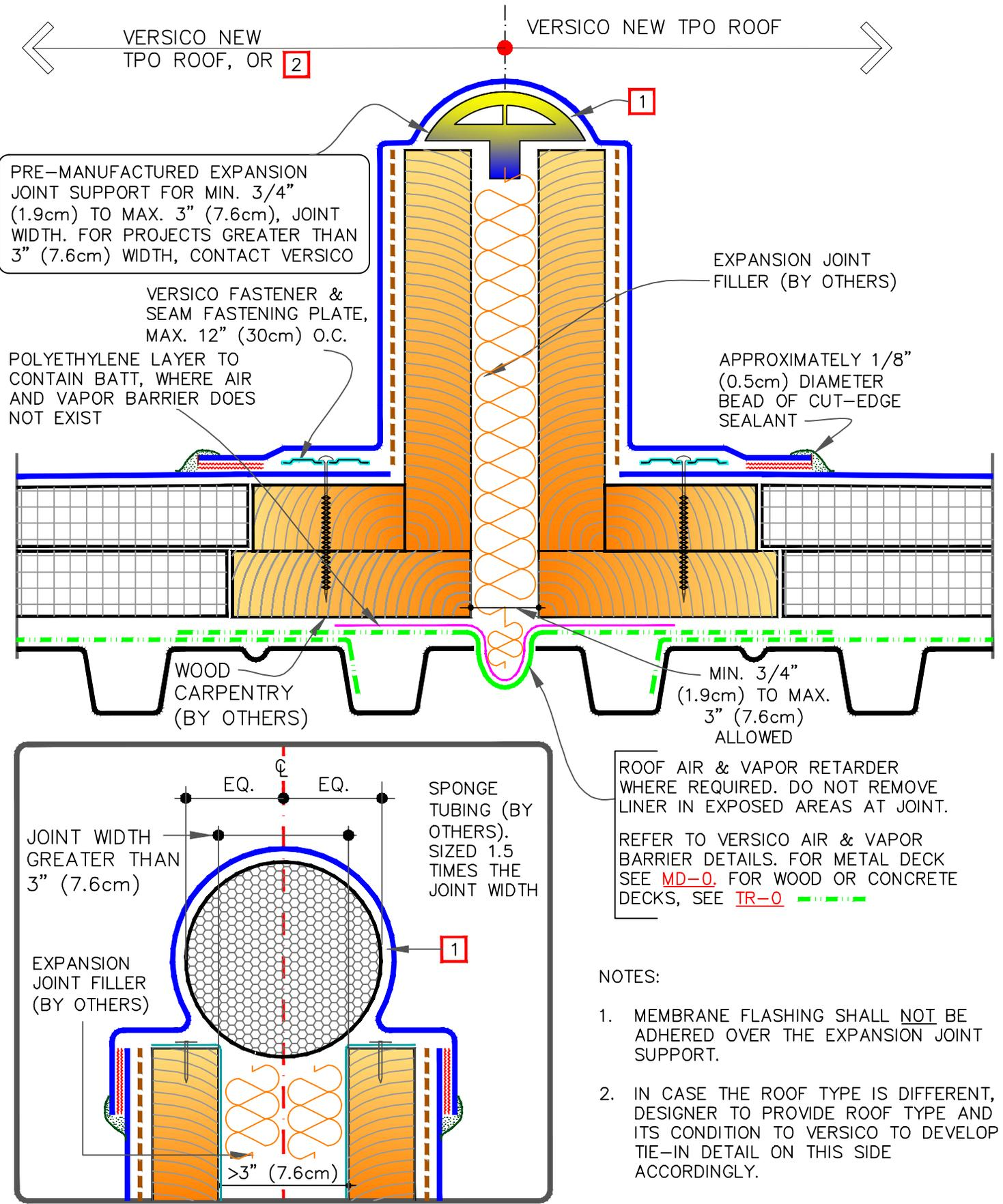
PRE-MANUFACTURED EXPANSION JOINT SUPPORT FOR MIN. 3/4" (1.9cm) TO MAX. 3" (7.6cm), JOINT WIDTH. FOR PROJECTS GREATER THAN 3" (7.6cm) WIDTH, CONTACT VERSICO
