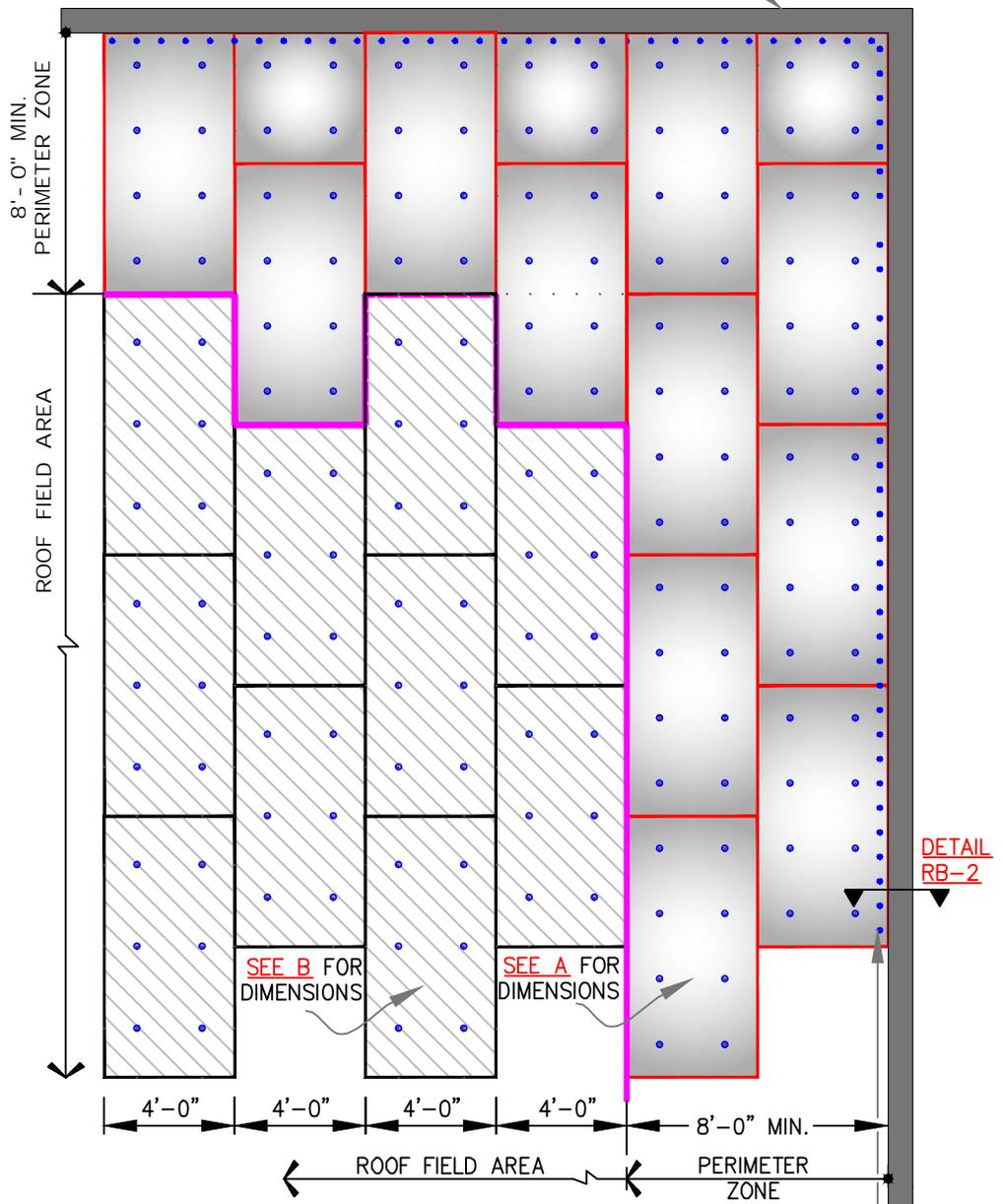
MEMBRANE FASTENED MINIMUM 12" O.C. AT ANGLE(S) CHANGES. FOR ADDITIONAL INFORMATION SEE DETAIL RB-2
