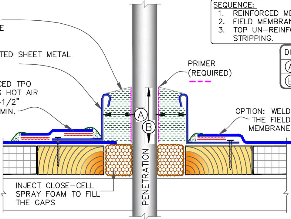
INJECT CLOSE-CELL SPRAY FOAM TO FILL THE GAPS
