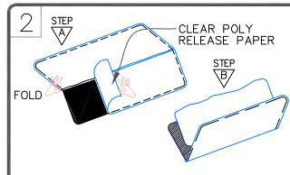
PRIOR TO PLACEMENT OF VERSIGARD WHITE PEEL & STICK VERSIGARD CORNER, PEEL OFF THE POLY RELEASE FILM FROM THE FLASHING SIDE AND HEAT WITH A HEAT GUN. RE-APPLY THE POLY LOOSELY. FOLD THE FLASHING IN HALF.
