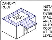
INSTALL PERIMETER SHEETS OVER THE ENTIRE OVERHANG (PROJECTION ROOF) AREA, EXTENDING ONTO THE MAIN ROOF DECK WHEN AT THE SAME LEVEL AS SHOWN.
