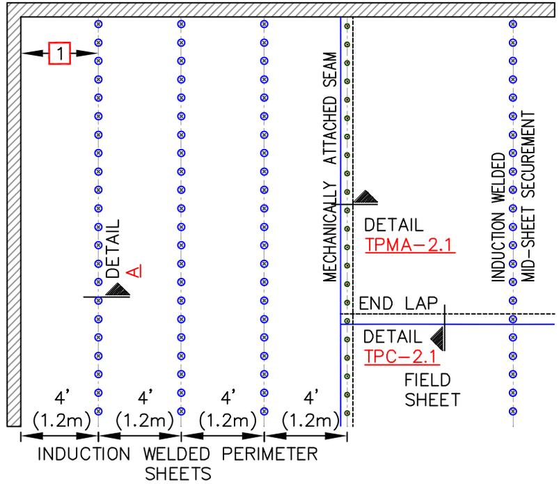
**PERIMETER SHEET SECUREMENT – FINGER METHOD**
