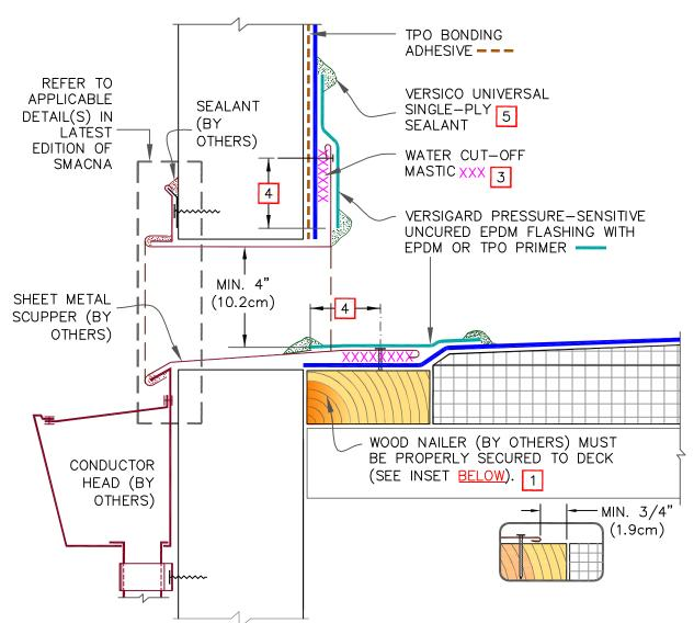
WOOD NAILERS ARE INSTALLED AT SCUPPERS TO SECURE METAL SLEEVE AND MUST EXTEND PAST THE WIDTH OF METAL SLEEVE FLANGE.
