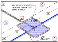
APPLY PRESSURE—SENSITIVE T—JOINT COVER OR 6" (15cm) WIDE SECTION OF PRESSURE—SENSITIVE ELASTOFORM FLASHING CENTERED OVER THE INTERSECTING POINT OF THE LEADING EDGES OF THE FIELD SPLICE INTERSECTION AS SHOWN.
