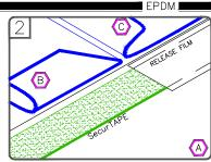
FOLD SHEETS BACK AS SHOWN. APPLY EPDM PRIMER TO THE SPLICE AREA ON BOTH SURFACES AND ALLOW TO FLASH-OFF. APPLY SecurTAPE WITH RELEASE FILM ALIGNED WITH MARKED LINE.
