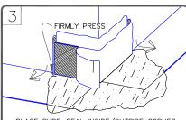
PLACE SURE—SEAL INSIDE/OUTSIDE CORNER AS SHOWN AND REMOVE RELEASE PAPER. PRESS FOLDED FLASHING TIGHTLY INTO ANGLE CHANGE AND FIRMLY PRESS FLASHING AGAINST THE VERTICAL SURFACE.
