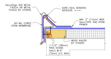
6" (15cm) WIDE PRESSURE—SENSITIVE ELASTOFORM FLASHING, IN CONJUNCTION WITH EPDM PRIMER, MUST BE CENTERED OVER FIELD SPLICES AT THE ANGLE CHANGE.
