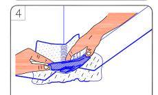
ROLL AND CREASE FLASHING TIGHTLY INTO ANGLE CHANGE AND FIRMLY ROLL FLASHING ONTO THE DECK MEMBRANE.
