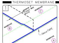
POSITION MEMBRANE TO ALLOW AN APPROXIMATE 4" (10cm) OVERLAP. MARK THE BOTTOM SHEET WITH AN INDELIBLE MARKER 1/2" (1.5cm) FROM THE EDGE OF THE TOP SHEET AS SHOWN. THE PRE-MARKED LINE ON THE MEMBRANE EDGE CAN ALSO BE USED AS A GUIDE.
