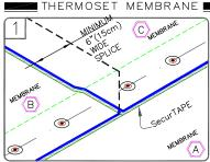
POSITION MEMBRANE TO ALLOW AN APPROXIMATE 7" (17.5cm) OVERLAP. THE PRE—MARKED LINE ON THE MEMBRANE EDGE CAN BE USED AS A GUIDE FOR TAPE PLACEMENT.
