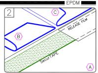
FOLD SHEETS BACK AS SHOWN. APPLY EPDN PRIMER TO THE SPLICE AREA ON BOTH SURFACES AND ALLOW TO FLASH-OFF. APPL SECURTAPE WITH RELEASE FILM ALIGNED WITH APPLY EPDM APPLY MARKED LINE.
