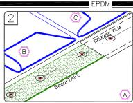
FOLD SHEETS BACK AS SHOWN. APPLY EPDM PRIMER TO THE SPLICE AREA ON BOTH SURFACES AND ALLOW TO FLASH-OFF. APPLY SecurTAPE WITH RELEASE FILM ALIGNED WITH PRE-MARKED LINE.
