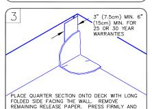
PROCEED WITH SECOND QUARTER GOING UP THE VERTICAL WALL BY PRESSING FIRMLY INTO CORNER.
