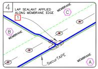
SPLICE SHEET C TO SHEET A AND B, PRESS TOP SHEET ONTO BOTTOM SHEET USING HAND PRESSURE TOWARDS THE OUTER EDGE OF THE SPLICE AND ROLL THE SPLICE AREA WITH A 2" (5cm) WDE STEEL ROLLER.
