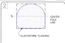
CUT A 9"x9" (23cm x 23cm) SECTION OF PRESSURE—SENSITIVE ELASTOFORM FLASHING AND MAKE ROUNDED CORNERS AS SHOWN.
