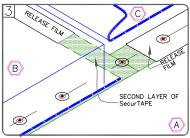
SPLICE SHEET B TO SHEET A AND APPLY SECOND PIECE OF SecurTAPE BETWEEN SHEET B AND C. TRIM RELEASE FILM AS SHOWN.
